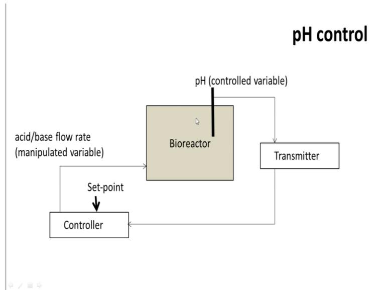
This schematic for pH control is something like this, pH is the controlled variable which is measured through the pH probe. The pH value which is measured electrochemically is sent to the transmitter, the transmitter to the controller, there is a set point which is optimal for the cultivation that is set here. Actions are taken to manipulate the acid or the base flow rate that is what is the manipulated variable here, into the bioreactor to maintain the pH at a preset value.
