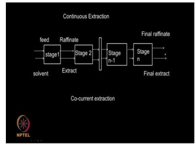
Analogous to counter-current we can also have a co-current that means both are flowing in the same direction okay and like the other one and you can prove that co-current operation is not efficient at all when compared to counter-current. I will leave it to you to prove that that co-current is not efficient compared to co counter-current at all. Okay let us go back to counter-current, so in a counter-current the feed moves in one direction, the solvent moves in another direction.
