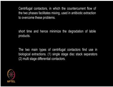
So there are contactors, I think in the previous class, we saw different types of contactors, the mixersettler type of contactor, then I discussed lot about the column type of contactors. That means vertical columns which occupies less space than centrifugal contactors is another approach, where you can get very high a mass transfer dispersion, so that the transfer of solute from the feed into the solvent becomes very facile actually.
