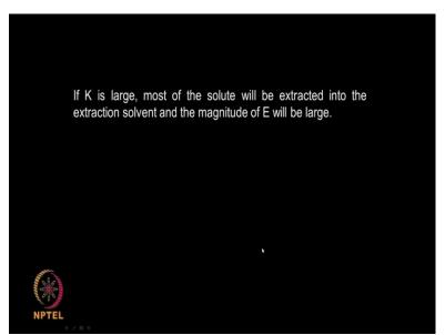
If K is large that means most of the solute will be extracted into the solvent okay. If K is large obviously your E will be large okay so the extraction efficiency will be also very large okay. (Refer Slide Time : 09:58)
