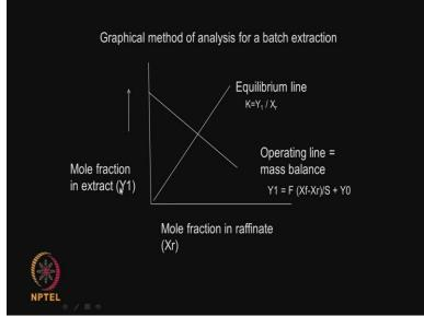
So what you do in graphical method, so in the first method, okay analytical method, if I know these terms like F S and K, I can calculate E and then I can substitute into this and then I can calculate, what will be the Xr so I can get the fraction extractor and so on. In the graphical method for batch extraction, we draw a graph where we have on the x-axis, the mole fraction in the raffinate okay and in the y axis we have the mole fraction in the extract.
