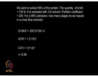
This is called cross flow. cross flow, what do you do? Every time you are adding the solvent, it could be fresh solvent or into each stage okay. So your feed flows stage 1, stage 2, stage 3, stage 4, whereas solvent is entering independently in each of these stages, that is called the cross flow extraction okay. (Refer Slide Time : 20:15)
