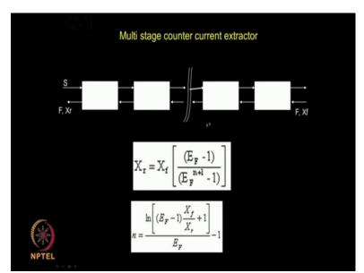
So there is a difference between the previous an this in cross flow we have Xr = Xf / e + 1 or 1 + E raised to the power 1 here the equation is different the assumption here, K is same in each stage that means it does not change irrespective of the concentration, K does not change. so K remains the same in all places okay. So I can adjust these equation to get into relation for n also that means if I want to find out how many stages I can do that also so this equation is very very important.
