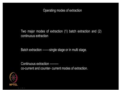
So operating mode of this extraction, it could be a batch or it could be continuous. Okay so the batch extraction could be single stage or multistage, continuous could be co-current or counter-current. Okay the in the single stage you may be adding fresh solvent in the multistage also you may be adding fresh solvent so you will look at each one of them little more in detail.
