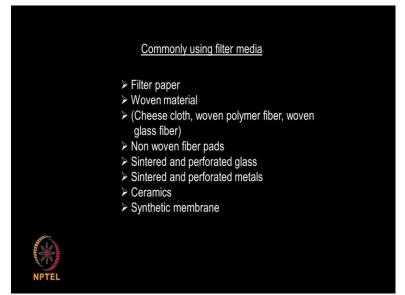
Commonly using filter medium, filter paper, woven material, cheese cloth, polymer fiber, woven glass, non woven material, sintered, perforated glass, perforated metal, ceramic, synthetic membrane, so almost anything can be used you can directly perform filtration at high temperature, room temperature and so on.
