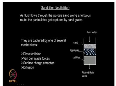
Depth filter that is called the sand filter or the depth filter so you have a bed pebbles which are of larger size then you have aggregate which are of smaller size then you have sand which are smaller
