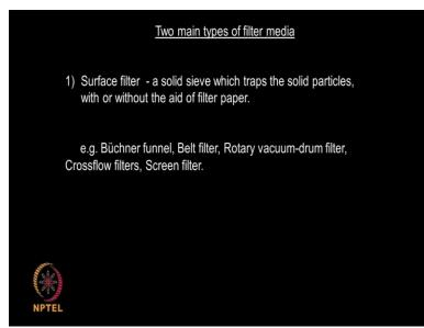
There are two types of filtrating system, one is called the surface filter. When you have a solid sieve or a solid piece of cloth or metal or ceramic like your Buchner funnel belt filter or rotary vacuum-drum filter all these come under surface filter. So the solids are retained on the surface, the liquid flows through, that is why the name is called solid surface filter.
