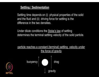
So particles have to be denser than the liquid. That is very very important and because of these density difference that gives you a driving force, so that settling time of the solid in this liquid, depends on the
