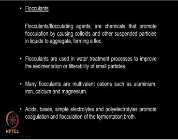
So there are flocculants that are used synthetic chemicals, natural chemicals and so on that are used to break this type of charges on that actually. They are generally used quite a lot in water treatment plant, they are used in environmental plant, when you are remediating the effluent that is getting discharged and so on actually. So what are these flocculants? They are generally multivalent cations like aluminum.
