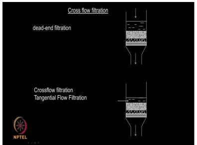
Now two types of filtration you need to know, the dead-end filter the liquid flows the slurry flows like this, so you have the cake that is formed at the top and the liquid is collected. So the problem in this type of filtration is, after sometime the cake thickness increases and increases and the flow of the liquid become negligible you need to stop it and you need to scrape off all the cake clear the top of the filter medium so that again the filtration can be started.
