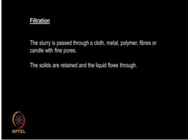
Okay now we saw sedimentation, we saw flocculation and so on now the next one is filtration. Okay you must have all seen filtration from very early ages, so the slurry is passed through a cloth, metal, polymer fibers or candles with fine pores solids get retained and liquid flows through (())(17:02) (Refer Slide Time : 17:05)
