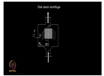
You have disk stack centrifuge, you have lot of disk here, okay so the liquid is flow the slurry is flowing from the bottom and it hits this angular disk and the solids get thrown out and the liquid flows upwards so that because of this the solids gets thrown out and hits the wall and they are collected at the corners of this wall. So the solids are collected at the corners at the walls the liquid flows through, so that is called the disk stack centrifuge because we have disks.
