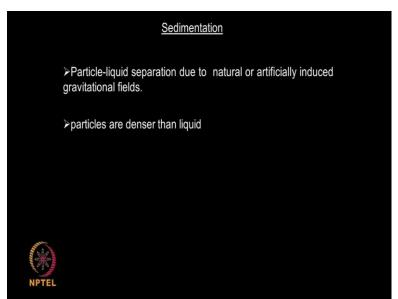
Okay so one of the easiest solid liquid separation is called sedimentation. Okay. So why does it happen? The solids settle down due to natural or artificially induced gravitational fields. It could be a natural gravitational field or it could be because of a centrifugal force, the solids could be separated actually.
