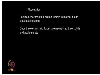
Flocculation, what is flocculation? Sometimes very fine particles, they do not settle down at all. That is because there are lot of electrostatic forces like particles with 0.1 micron, they always remain away from each other because of this electrostatic forces. So they do not agglomerate at all. So you want to separate them. Filtration may be a difficult option because the particle sizes are very small, so you resort to something called flocculation or agglomeration.
