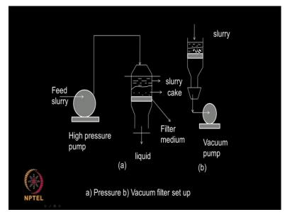
So this is generally used in water treatment even in households you may see. Okay so you can have pressure type of filtration, you can have vacuum type of filtration here. So pressure means this slurry is forced on top of the filter medium under pressure whereas in the vacuum, a vacuum is used at the bottom so that the slurry is sucked, the solids are retained and the liquid goes down and so both the techniques are commonly used the pressure type and vacuum type.
