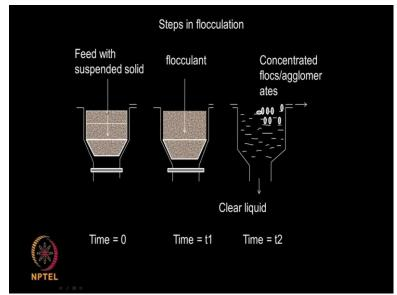
Now analogous to that, if the flocs are lighter than the liquid, then it may float. So at time equal to 0 you take your feed, then you add your flocculant at time equal to t1 and then after sometime the solids which are floating or skimmed off or removed at the top and the liquid is at the bottom just clear so both the approaches are possible depending upon the flocs that are formed later or heavier or lighter
