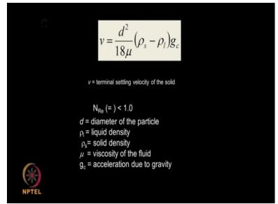
So you have to balance all these forces and you end up with the new equation like this. The terminal settling velocity = d square. That is the diameter... d is the diameter of the solid, Mu is the viscosity of the solid, row s is the density of the liquid, solid sorry density of the solid and row l is the density of the liquid and you have the g the gravitational force. Okay so the velocity, that is the terminal settling velocity depends upon the solid.
