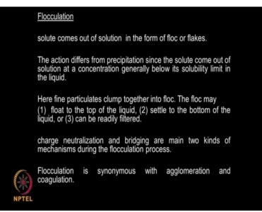
So you can remove it as a flake or it can be like a flock, like a precipitate basically but there is a difference between precipitation and flocculation. In precipitation, the concentration is larger than the solubility of the solid in the liquid. That is why it precipitates whereas in flocculation, we have finely divided solid present inside the liquid, they are not coming together because of the electrostatic operations.
