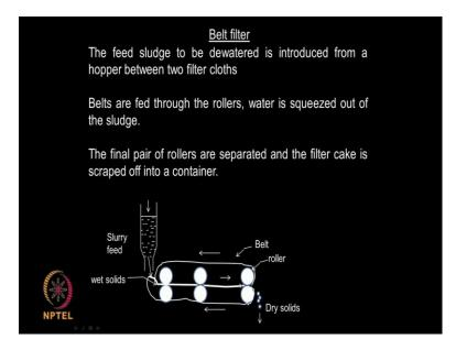
Then you have this belt filter, what happens is, this is a long belt this can be hundreds of feet long and the feed slurry is charged here okay, the feed slurry is charged here and then the it moves along between two rollers okay so the water is squeezed out as you go through these rollers actually. There are 2 different belts and the solid is between is these rulers and because of these rollers, the water gets squeezed out and then at the end of it the dry solids fall off.
