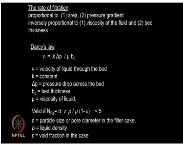
Now generally filtration is based on Darcy's law. We are going to spend some time on Darcy's law and this is what filtration is based on. Where the velocity of flow of the liquid through the bed is directly proportional to the pressure difference inversely proportional to the viscosity and v d is the bed thickness. So the bed thickness is higher and higher your velocity goes down if the bed thickness is lower and lower the velocity goes up.
