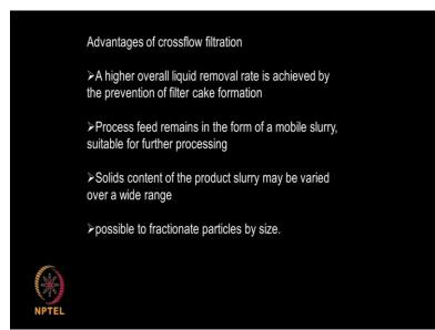
What are the advantages of cross flow? The liquid removal rate, a good liquid removal rate is achieved because you are not allowing it to form large thick cakes and in a dead-end thick cakes make the liquid flow less and less and after sometime the liquid flow can totally stop actually. And the feed always keeps moving on top, so we can take it and do further processing unlike thick cake thick and dry cake where we cannot do further processing unless you put it again in a slurry.
