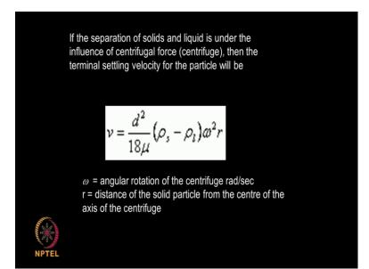
When you have settling taking place in a centrifuge, then instead of g which is the gravitational force, you will have omega square r. Okay what is the omega square r? Omega is your angular rotation of the centrifuge, that is radiance per second, R is the distance of the solid particle from the center of the axis okay. Further the particle away from the center going to have high driving force. That is why you have r here and larger is your rpm, larger will be your settling velocity.
