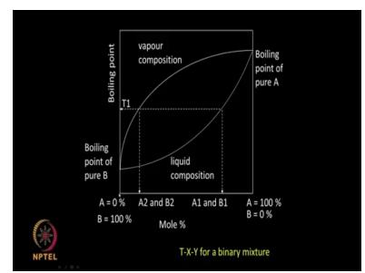
So you can also plot the concentration of A in the X-axis and we can plot the vapor composition, that is the composition of A in the vapor and composition of A in the liquid. So you can have graphs like this so this could be boiling point of pure A and this could be boiling point of pure B so A at 0 % here A at 100 %. So here you have B at 0 % B at 100 % so this is the composition of A in vapor phase this is the composition of B in the liquid phase.
