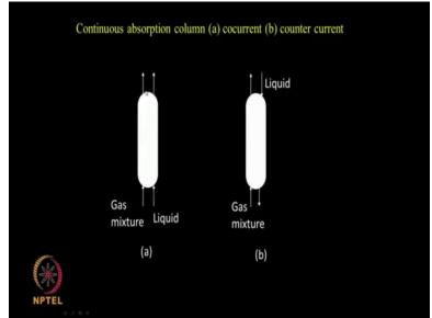
Generally the adsorptions are done in tall tower of columns, okay so you have the gas mixture going in okay and the liquid also going into the column either in co-current or counter-current manner and they to the gas is vented out at the top and the liquid is collected at the bottom. So in the counter-current, the liquid enters the liquid could be water or amenical solution or alkali and A gas that needs to be scrubbed comes from the bottom rises and then it goes out.
