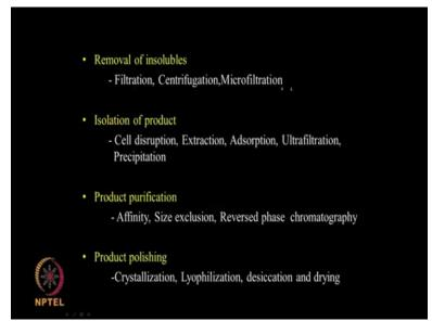
So we have removal of insoluble, which may include filtration, centrifugation, microfiltration, some membrane operation then we have the isolation of product, cell disruption, adsorption, ultra filtration, precipitation. Then we have the product purification chromatography, affinity chromatography, size exclusion chromatography, reversed phase chromatography, then finally product polishing it could be crystallization, lyophilization, desiccation, so the product is drying.
