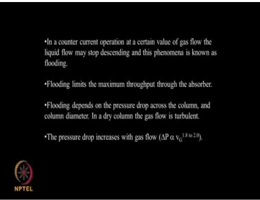
So in a counter-current operation at a certain value of gas flow, the liquid flow may stop descending and that is what is causing the flooding. So the flooding limit is the throughput, so the flooding depends on the pressure drop across the column, column diameter and so on actually so if I have a larger column, I will be able to prevent this type of planning. So the pressure drop
