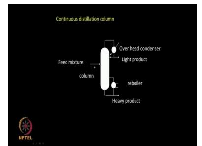
You can have a continuous distillation column, you are continuously introducing feed, the liquid will come down. This liquid will have more heavy product, vapor will rise. The vapor will contain more of light product which is collected here, the heavies are collected here. So continuously you are feedings something continuously, you are collecting light and continuously you are removing heavies this is A continuous distillation column.
