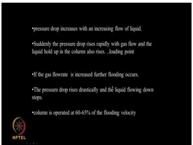
Okay so pressure drop increase with the increase in fluid and suddenly the pressure rises rapidly reaching A loading and then the flooding. Okay. The columns are operated generally 60 to 65% of the flooding velocity.
