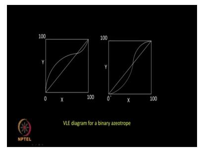
So if you look at the VLE diagrams corresponding VLE diagrams, for azeotrope will look like this. Okay instead of the graph going either up or going down the graph will cross the 45 degrees line. So at this place or at this place the composition of the solute A will be the same into the liquid and in the vapor phase. So if you have this composition, you will not be able to separate by just boiling at all. So they are called constant boiling azeotrope
