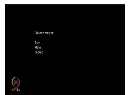
So the distillation columns can be tray, that can be plate, it can be packed column, even absorption column which I talked about few minutes back, can tray plate and packed. The idea of these is to bring the vapor and liquid into intimate contact so that there is A separation taking place.
