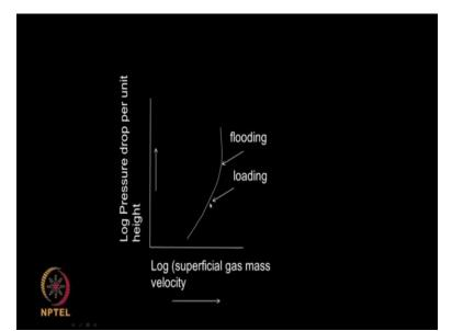
So you can keep on increasing the flow rate of the gas but then you cannot do that too much after sometime the gas velocity will be too high that it will prevent the liquid flowing down and that is called flooding. Okay these are very chemical engineering terminologies. So I need to operate my gas velocity much lower than this flooding velocity. Because if my gas velocity is too high, the liquid will not flow down. So the whole column will come to A standstill, so in the X axis.
