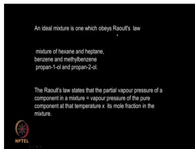
So ideal mixture is one which obeys Raoult's law in distillation there is Raoult's law. Like Henry's law in absorption okay, the Raoult's law states that the partial vapor pressure of A component of A mixture is equal to the vapor pressure of the pure component, at the temperature multiplied by it is mole fraction in the mixture. Okay will come to that so mixtures of hexane and
