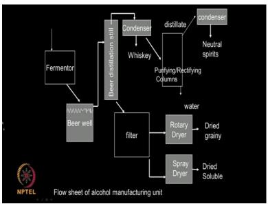
So here, this is an example of a flow sheet of a alcohol manufacturing process okay, as you can see on the left hand side, here the fermenter that is the heart of the entire unit operation, where the fermentation takes place okay. Once the fermentation is over, the product comes down and there is a distillation which happens here okay and the product ethanol is collected here on the top whereas the bottom contains all the solid material which is dried here and then it goes as a dried product.
