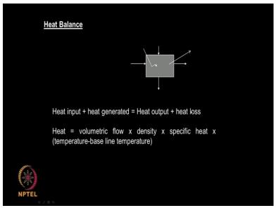
So we say heat input + heat generated is equal to heat output + heat loss. That is what is heat balance is all about. So if you have two streams, there will be two heat inputs. If you have two streams going out, there will be two outputs and if you have ten stream inputs then we will have to calculate the heat input for all the ten streams and if there are ten streams going out you will have to consider the heat output from all the ten streams.
