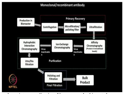
Now let us go further down into complication. Now we are looking at the monoclonal recombinant antibody, so in that as you can see after the bioreactor, we have the primary recovery and then we have the purification and then final filtration so initially again we have a centrifuge and then we
