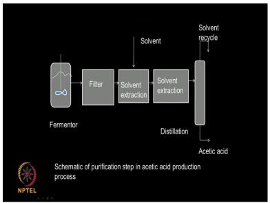
So if you look at here you have again on the left hand side, the fermenter then the filter. If you recall earlier I said that filter is the first downstream process after a fermenter or bioreactor to remove this solids, the biomass and then it goes into the extraction, you have a solvent and you have a dryer or extractor here, where the acetic acid is extracted with the solvent. And then again you have a distillation column where you get the pure acetic acid at the bottom.
