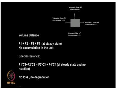
So if you are doing a volume balance F1 and F2 are the streams entering, F3 and F4 are the streams leaving. So F1 + F2 is equal to F3 + F4. So there is no accumulation inside the unit at steady state. Now if we do a solute balance, what do I do? F1 into C1 + F2 into C2 is equal to F3 into C3 + F4 into C4, there is no accumulation this is at steady state. So if I have two solutes then I will do species balance for solute 1, then I will do species balance for solute 2.
