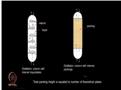
I want to introduce some new terminology theoretical plates. I introduce this terminology in the previous class. It a chromatographic column can be expressed in terms of theoretical plates, which gives a quantitative measure of its efficiency or separating part. How did this theoretical plate come? It came from chemical engineering. So if you look at an original distillation column
