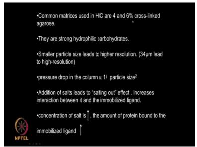
Common matrices used in HIC are 4 to 6 % cross-linked agarose. They are strong hydrophilic carbohydrates. Smaller particle size leads to higher resolution you know but then pressure drop also increases because pressure drop is inversely proportional to 1 by particle size square. So that problem we need to... Addition of salt leads to salting out. So increases the interaction between the protein and the immobilized ligand. So I can have a very high solvent.
