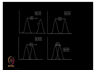
So resolution, this is how it looks like. Okay these peaks are very well dissolved, okay. So you can have this is almost at a distance of six sigma resolution may come out to be 1.5. So resolution 1 means they are just touching each other at the base and as the resolution keeps going down this starts slowly overlapping. So when poor resolution almost 0.5, we can see large overlap between these two peaks okay.
