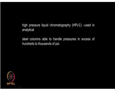
You all HPLC that is the high pressure, high performance liquid chromatography. Generally they are used for analytical purposes, they are not generally used for separations in industrial scale because they are very small diameter. So sample injection is very limited in this actually. (Refer Slide Time : 16:02)
