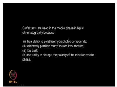
Surfactants are used because in the mobile phase, if you want to recover whatever has been because surfactants have the ability to solublize hydrophobic compounds. They selectively partition many solution to micelles cheap and it can also change the polarity of the mobile phase by adding that.
