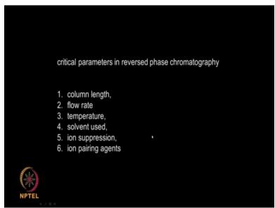
So what are the parameters column length flow rate temperature solvent used ion suppression sometimes, if the proteins has ionic groups then, it will appear like a polar. So we need to suppress that, so the hydrophobic part gets interacted with the stationary phase. So we need to have some ion suppressing agents, sometimes you need to add ions varying agents also basically. These are done to suppress the ionization of the protein.
