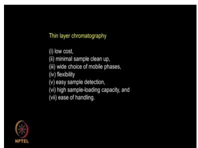
Okay there is something called Thin Layer Chromatography. This is we do it on a piece of glass plate which I coated by silica. So it is very cheap, minimal sample clean up, wide choice of mobile phases, flexible, easy sample detection, high sample detection, ease of loading. This is widely used in chemistry, synthetic labs for a very very long time, which it can be used for small molecules. It can be used for larger biopolymers as well actually.
