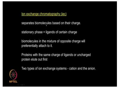
It separates biomolecules based on the charge, stationary phase ligands of certain charge. So it is all based on charge biomolecules in the mixture of opposite charge will attach to it, whereas with the same charge. It will pass through obviously right. So we can have cation and anion. (Refer Slide Time: 21:17)
