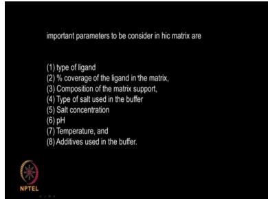
So important parameters I need to consider the type of ligand, percentage coverage of the ligand in the matrix, composition of the matrix, type of salt used, salt concentration, pH, temperatures, any additives that are being used and so on actually.
