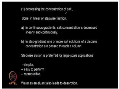
Decreasing the concentration of that salt can be done in linear or step wise fashion continuous gradient salt concentrations decreased linearly and continuously. Step-gradient one or more salt solutions of a discrete concentration are passed through a column okay. Step wise is simpler easy to perform reproducible. So water as an eluant also leads to desorption that means water without any salt right.
