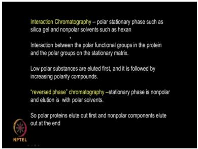
So interaction chromatography polar stationary phase like silica gel and non polar solvents like hexane whereas reversed phase chromatography stationary phase is non polar and elution phase is polar solvents like water.
