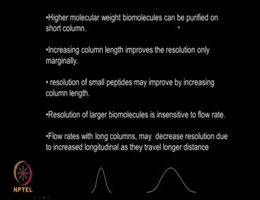
Higher molecular weight biomolecules can be purified on short column, increasing column length improves the resolution only marginally, resolution of small peptides may improve by increasing column length. Resolution of large biomolecules is insensitive to flow rate. So if I am doing flow rate with long, it may decrease resolution due to increased longitudinal diffusion as it travel longer. So if I have a small column, you may get like this.
