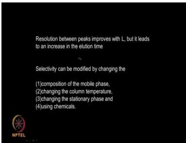
So the higher the resolution further away are the two peaks okay, the resolution between peaks improves with the length of the column but the problem is, if we increase the length, the illusion time also increases. The selectivity can be modified by modifying the composition of the mobile phase, changing the column temperature, changing the stationary phase, using some chemicals and so on actually.
