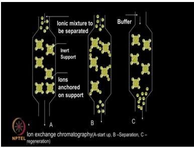
Now let us look at something called ion exchange chromatography. Okay. So basically if you have a ionic mixture, like you have a positive and negative okay, so we have a packed column okay which has ei either positive ion anchored on the support or it could be negative ions and sometimes it can have mixtures also. So what happens when you pass ionic mixture, okay, so the negative ions will get captured on the ions which are anchored.
