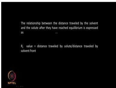
The relationship with the distance traveled by the solvent and the solute after they have reached equilibrium is expressed as Rf value. That is distance traveled by the solute / the distance traveled by the solvent front. Okay. So that is called the Rf value. So each component will have the Rf values and that is very characteristic of the component.
