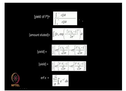
Then we can, the amount eluted out will be given by this, okay because c is given by this relationship as you shown before. Okay. So we can substitute in that and we come up with a new function that is called erf. erf is called error function okay, I will define that more in detail later on. But this is called error function, so yield is given by half of error function of t/t0-1 / square root of 2 \* sigma - error function t'/t0 - 1 /square root of 2 sigma okay.
