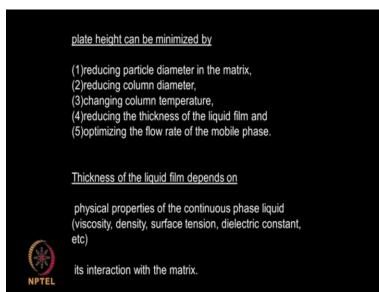
So there are different ways, by which one can calculate the number of theoretical plates using width at the base or width at the 10 % of the height or width at half the height and so on. So there is something called plate height. So if you have number of plates, then you have plate height. If you multiply together, that will give you an idea of the length of the packed portion. So plate height can be minimized by reducing the particle dia.
