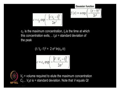
So if you assume a Gaussian distribution, then the as a function of time will appear like this. It will be c0 exponent t/t0 - 1/2 sigma square, t0 is called the retention time, c0 is the maximum concentration, the solute will appear okay and t0 sigma is the standard deviation. You can compare this equation with the normal Gaussian function, as you can see know, x-b the whole square / 2c square okay. So that is how it looks. That is how its analogous.
