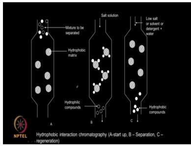
Next one is hydrophobic interaction chromatography. We looked at ion exchange. So in this hydrophobic interaction, we are separating proteins based on their hydrophobic nature of the surface. So I will have matrices which are hydrophobic. Okay. So what will happen proteins which are hydrophobic will get bound and proteins which are hydrophilic will get flushed out okay.
