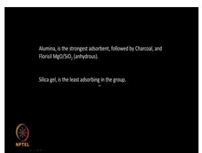
Alumina is a strongest adsorbent followed by charcoal and so on... silica gel is the least adsorbing in the group okay.
