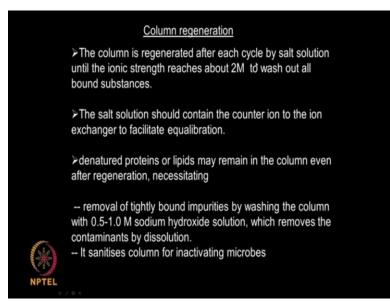
So this is how you regenerate your column. You have to regenerate after each cycle, you can use the salt solution. Until the ionic strength reaches about 2 molar, the salt solution should contain the counter ion to the ion exchanger, so that there is equilibration takes place. There could be denatured proteins or lipids which may remain in the column even after regenerating okay. So we need to wash it then with sodium hydroxide solution, so that the contaminants get roved actually.
