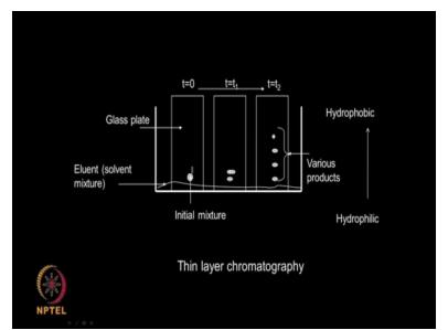
So basically what you do? We have a glass plate, we coat it with the silica and then you put an initial mixture of your the mixture and then you have a solvent here, could be a mixture of solvent. As time progresses the spot keeps moving up, as you know silica is extremely hydrophilic. So it does not move, whereas hydrophobic material keeps moving. So as time progresses and progresses, you are going to have many spots depending upon the optimization of the sol mixture of solvents.
