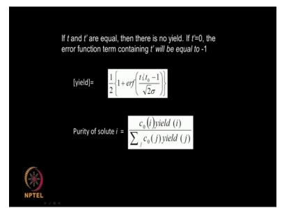
So this table is very important if I want to calculate for example yield. If I am collecting samples from 0 time to time t I use this equation. So I will calculate all these terms and error of x whatever is this, then I go to the table and pick up my corresponding value okay and that is how it works.
