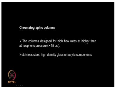
The columns designed for high flow rates are higher than the atmospheric pressure. These columns are stainless steel or high density glass or acrylic components. These are the chromatographic columns are made actually.
