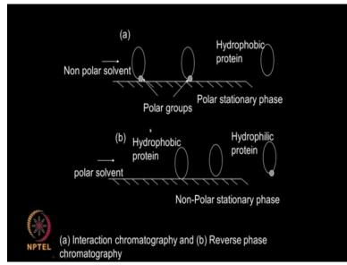
There is interaction chromatography. So this is you are looking at polar stationary phase. Okay. Then you are using a non polar solvent, okay non polar solvent. What is a non polar solvent? It could be a hexane could be toluene and so on...So polar stationary phase this is a normal chromatography. Whereas if you look at the reverse phase chromatography, you have a non polar stationary phase. That is the hydrophobic interaction chromatography and you are having a polar solvent.
