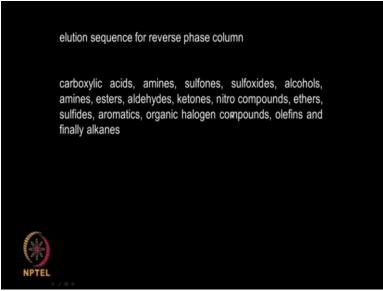
So elution sequence for reverse phase carboxylic acid, amines, sulfones, sulfoxides, alcohols, amines, esters and so on actually and finally the alkanes are there actually.
