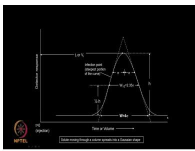
We will continue on the topic of chromatography. So as I mentioned that the peak that is coming out of the column will appear like a normal distribution or a Gaussian distribution and you have the width at the base and this is called the half width at half the maximum. Okay. This is the width at half the maximum. These parameters are used quite a lot, for doing some calculations which we will see that later.
