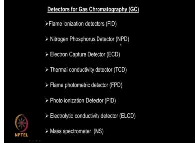
Similarly detectors for Gas Chromatography, We Can Have Flame Ionization Detector, Nitrogen, Phosphorous Detector, Electron Capture Detector, Thermal Conductivity Detector, Flame Photometric Detector, Photo Ionization Detector, Electrolytic Conductivity Detector, Mass Spectrometer and so on. So large number of detectors depending upon type of compounds you are separating whether it is ionizable non ionizable, whether it is ui visible, all those things actually.
