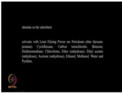
Alumina as the adsorbent, then you use different solvents for these solute mixture to travel upwards right. So you can have Petroleum Ether And They Have The Least Eluting Power And They Have Cyclohexane, Carbon Tetrachloride, Benzene, Dichloromethane, Chloroform Ether, Ethyl Acetate, Acetone, Ethanol, Methanol, Water And Pyridine. So if alumina is the adsorbent, then least eluting power solvents are given in that order.
