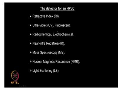
So what are the detectors? The HPLC detectors could be Refractive Index Detector, Ultraviolet Fluorescent Detectors, Radiochemical, Electrochemical, Near-Infra Red Mass Spectrometer, Nuclear Magnetic Resonance Light Scattering. So large number of detectors can be used. We will not spend time on those because we have shortage of time.
