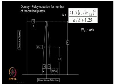
So the tailing factor is defined by a + b / 2a. What is the front portion of this is called a and the back portion is called b okay. So the tailing factor tf is a + b / 2a. Generally this factor will vary
