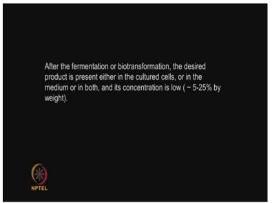
So after the fermentation or biotransformation, the product that is the desired product is present either inside the cells or in the medium. So sometimes your product is inside the cells that is called intracellular product. Sometimes the product is in the liquid medium that is called the extracellular. Okay. So you would like to consider both, whether it is intracellular or extracellular and that is what you are trying to recover.
