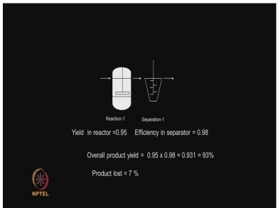
So let us look at very interesting problem here. Okay. Suppose there is a bioreactor or there is a fermenter where the yield in the reactor is 95% that is 0.95. Okay. You take the fermentation broth and you have one separator and efficiency of the separator is 98% that is 0.98. So what will be the overall product yield do you think? So yield in the reactor is 95%, the efficiency of the separation is 98%. So what will be the overall product yield?
