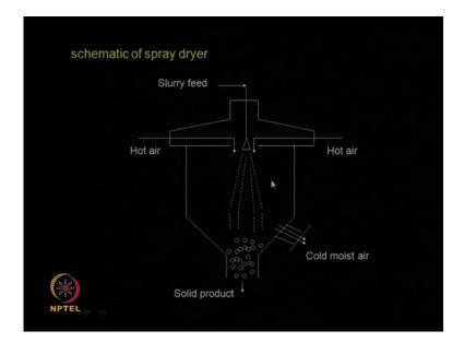
So, how does it look like so this is a typical setup of a spray dryer so you are feeding a slurry to the top, it comes out through the nozzle as a fine spray. We have hot air coming in contact, so your solvent for water gets evaporated, so fine microns size particles are
