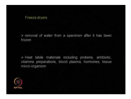
Freeze dryers, now the previous dryers where, you are applying heat or temperature to raise the temperature of the solid and the vapour. Whereas here, you are using the freezing concept that means, you are reducing the temperature so that, the moisture becomes ice. So, water is removed after it has been frozen, it is very very good for heat labile materials like proteins, antibiotic, vitamins, blood plasma, hormones, tissue, micro organisms.
