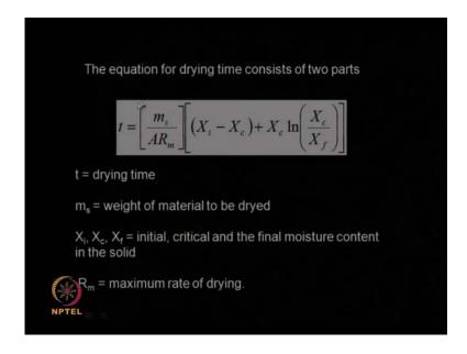
Now, based on that and also we said, that there are two types of regions, one is the constant rate drying and falling rate drying. We have a mathematical relation, which relates the drying time t to many other parameters so t is made up of the weight of the material that needs to be dried, A is the area of the surface area, R m is the maximum rate of drying, X i is the initial moisture content, X c is the critical moisture content, X f is the final or the equilibrium moisture content.
