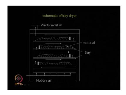
So, there is a typical schematic of a tray dryer so hot air is coming from the bottom so how do you heat air, there could be a external heater electrical or it could be a hot water heating up the air and it could be a dehumidifier. So, this air comes in contact with the solid material, which is placed on trays so the travel through the porous solid material there by carrying the moisture as well as drying the material.
