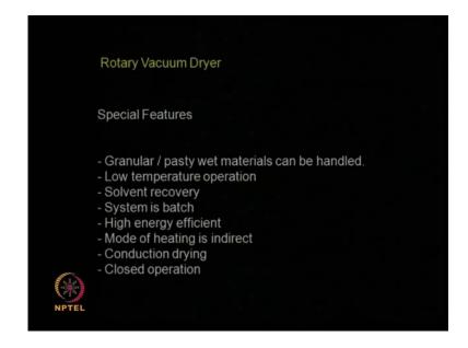
So, this dryer is very, very common, if you go to a pharmaceutical company you may find this type of dryers. It is very good for granular pasty wet materials, it is very good for low temperature operation and it is very good for solvent recovery. And we can do it in a batch and it is also very high energy efficient, the mode of heating can be indirect or it can be even direct.
