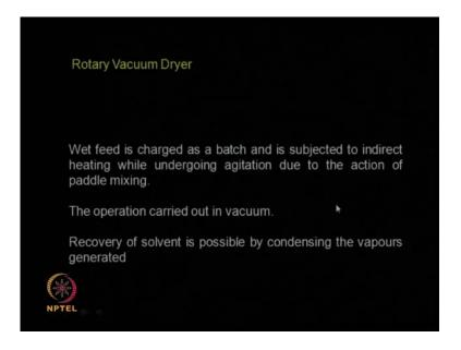
You have the rotary vacuum dryer so you have the drum rotating, there is a vacuum applied inside the drum, the drum surface is maintained at high temperature. So, the wet field is charged as a batch and is subjected to indirect heating and it is undergoing agitation due to the action of the paddle mixing. So here, you can carried out the
