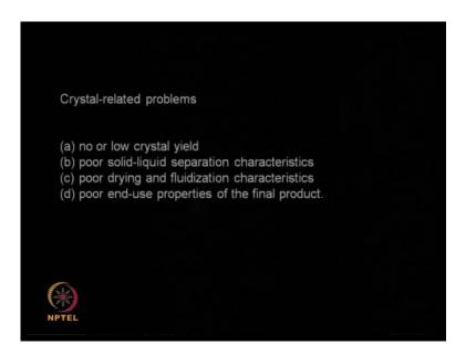
So, the crystal related problem leads to: low crystal yield, poor solid liquid separation, poor drying and fluidization. That means, after your crystallization you are not able to dry fully or poor end use properties. That means, the final product is not having all the properties of the real solid because of some impurities or because of removal of solvent or because of the type of crystal that is formed and so on.
