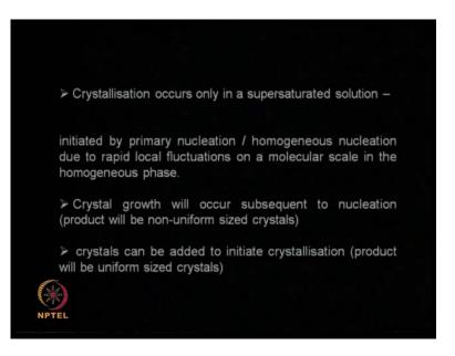
Now, let us go back again to the engineering side of it. So, crystallization occurs only in a super saturated solution. You need to have a primary nucleation that is homogeneous nucleation due to fluctuation on a molecular level or we can induce by adding very fine particles. That means, we can add to initiate crystallization but when it is happening because of nucleation then your product will be of non-uniform sized crystals.
