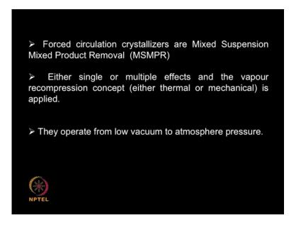
So, they are also called mixed suspension mixed product removal. As we can see its suspended, you are removing product combination. We can have single or multiple effect. I will talk about what is a single effect and in multiple effect later. It can have a different types of recompression that means vapor can be recompressed using thermal or mechanical approach.
