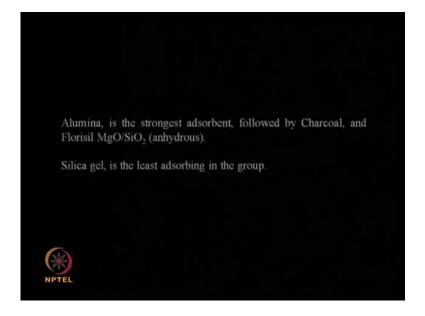
So, alumina is the strongest adsorbent followed by charcoal and florisil, magnesia, silica anhydrous and so on. Silica gel is the least adsorbing in this particular group of components actually.
