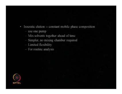
There is something called isocratic elution that means I use only one mobile phase. It is very simple, very cheap I use only one solvent, I use only one pump. The pump is very very expensive in a HPLC. Now, using only one pump and able to bring down the cost or if I want to use two solvents, I mix the solvents and make it in a container and use that mixed solvent for elusion.
