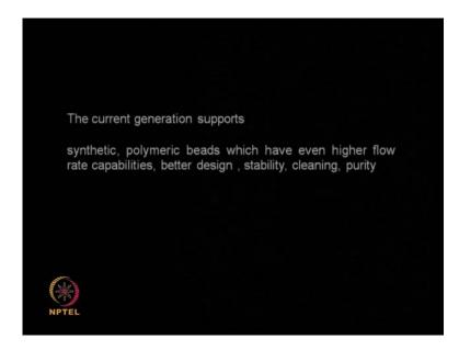
Then as time moved on they went into synthetic polymeric material, polystyrenes and different types of polymers because we can achieve very high flow rate, we can have good designs, stability it is easy to clean and we can achieve very high purity, so currently only polymeric stationary phases are used.
