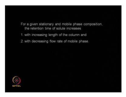
For a given stationary phase and mobile phase, the retention time of the solute increases with increasing length of the column it is obvious. So, if I have a longer column it takes much longer time for the sample to come out so this is obvious. The retention time of the solute increases with decreasing flow rate of the mobile phase. So, if the flow rate of the mobile phase is low obviously, it takes much longer time for the solute to come out. So, both these statements are very true and obvious.
