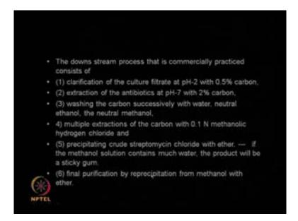
So, what are the downstream steps that are commercially practiced? First is the clarification of the culture filtrate. So, clarification means, you are removing the flocculants so it is based on pH adjustment you and it uses carbon to absorb the
