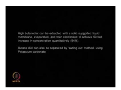
You can also use solid supported liquid membrane for extracting and then later on you can remove the liquid membrane. So, that the Butanediol is extracted. So, this is very good process you can extract almost 95 percent 94 percent of the Butanediol. You can also use a salting out technique by adding potassium carbonate. So, I add potassium carbonate so because of the changes in this solubility Butanediol precipitates out.
