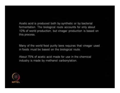
So, acetic acid can be manufactured both by synthetic root as well as the bacterial
