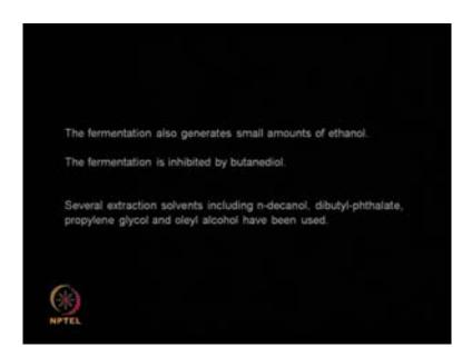
The fermentation also produces little bit of ethanol that is one point. So, ethanol Tolerancy is very very important number1, number 2 Butanediol itself is toxic to these organism. So, what you have to do is as soon as you produce Butanediol you have to remove the Butanediol and then send, and then brought back into the reactor for further fermentation.
