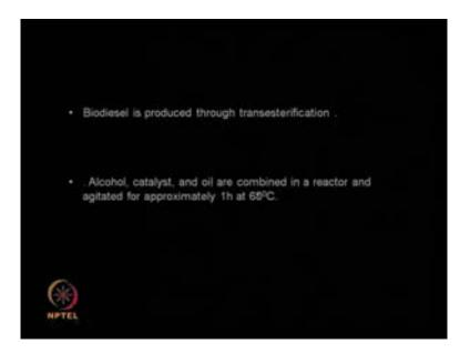
So, this is a Transesterification reaction. So, the methanol reacts with the trigliseride and then it produces a methyl ester that is; why it is called a transesterification reaction. So, the reactor will contain an alcohol that is; methanol, a catalyst and the vegetable oil. Generally, the reaction takes place within 1 hour and you use about 60 to 70 degrees temperature.
