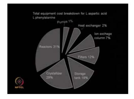
Again, if you look at L-aspartic acid, L- phenylalanine reactors take up 31 percent of the cost, crystallizers take up 21 percent of the cost, storage tank takes up 19 percent of the cost and filter takes up 12 percent of the cost. So, reducing the size of the filter, storage tank and crystallizer one can really bring down the total equipment cost in the manufacture of aspartic acid and phenylalanine.
