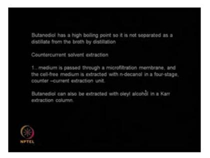
So, Butanediol has a very high boiling point. So, you cannot use a distillation column and hope to get Butanediol at the top of the distillation assembly. So, that is the main problem; so extraction is the only way of extracting Butanediol after the fermentation. So, how do you do it? First the medium is passed through a filtration membrane so once it passes through the cell free medium is obtained.
