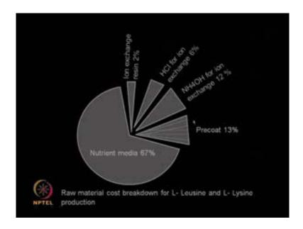
So, this is a picture which tells you the raw material cost break down for the manufacture of L –Leusine and L- lysine. So, 67 percent of the cost is because of the nutrient media; so you can focus on optimizing the nutrient media. A typical nutrient media will contain a carbon source, a nitrogen source, micro nutrients, salts, metals and so on. So, if you can reduce the usage of the obviously you can impact this cost.
