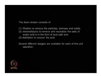
So, what are the down streams? So, once you make the acetic acid you have to filter the media. So, for removing the particles, biomass and solids and then you resort to electro dialysis to remove and neutralize the salts that are present because you are going to have lot of salts present. So, that the acetate becomes acetic acid and then finally, you resort to distillation to recover the acid.
