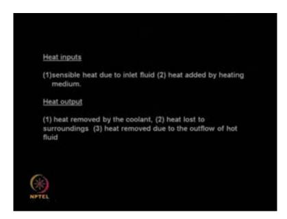
So, the heat inputs as I said is sensible heat due to inlet fluid, heat added by heating medium or exothermic heat. And then heat removed by the coolant, heat lost the surroundings or heat removed due to the out flow of the fluid. The outflow of the fluid is like this these 2.
