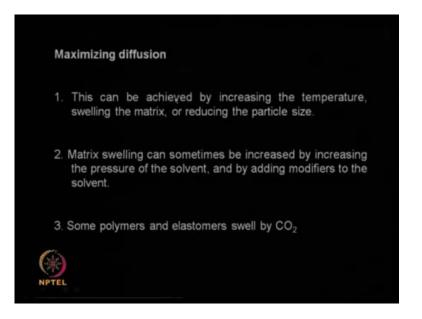
If you are talking about optimization we need to also consider the improving the diffusion. So, this can be achieved by increasing the temperature, assuming that the chemicals that are getting extracted, do not get degraded at higher temperature swelling the matrix. So, if you have a solid plant material or if you have a solid food product, by swelling it you can allow the fluid super critical fluid to enter through the interstices, small pores and, so on.
