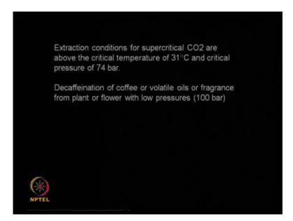
So, what are the extraction conditions for super critical CO 2 for example, I can the critical temperature is 31 degree centigrade, and critical pressure is 74. That means, if I am above this temperature, and above this pressure CO 2 will be in the form of a super critical fluid. And I can process any system, and by modifying the pressure I can improve the solubility's, and I can modify the temperature to improve the diffusion coefficients.
