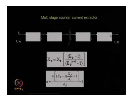
Now, let us look at another problem, this is a multistage counter current extraction; that means, the solvent is flowing in one direction, your feed or the heavies is flowing in another direction, that is why it is called a counter current. The solvent when it is entering it is devoid of any solute, so the concentration of solute in the solvent layer is 0. Now, feed is entering at solute concentration of X f and the raffinate that is leaving on the other end has a concentration of X r.
