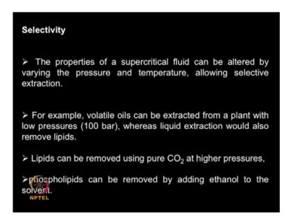
So, we can change the selectivity by changing the pressure and temperature for example, volatile oils can be extracted from a plant, at a pressure of a 100 bar whereas, if you are using a liquid like hexane, it may also remove a lipids. So, super critical fluid that way can be very selective I can use CO 2 at very high pressure to remove lipids alone, and I can remove phospholipids by just adding ethanol to the solvent. That means, you are adding entrainer to this super critical CO 2.
