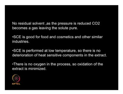
Main advantage here is I can reduce the pressure, and convert the super critical carbon dioxide into the gas. So, there is no residual solvent left behind with the solute, so the solute will be 100 percent pure, so it is good for food and cosmetic and other similar industries, cosmetic industry also love super critical. Because, in a normal cosmetic industry they use to use ethanol, pentane, ethyl acetate that sort of solvent, so you need to select solvent which are not toxic to human.
