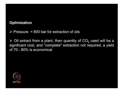
So, if you are talking about extracting oils I may go up in pressure because, if you take an oil extraction plant, then the quantity of CO 2 used will be a significant cost and complete extraction might not be required even a yield of 70 to 80 percent is economical, and the most of the cost is because, of the quantity of CO 2 that is used actually.
