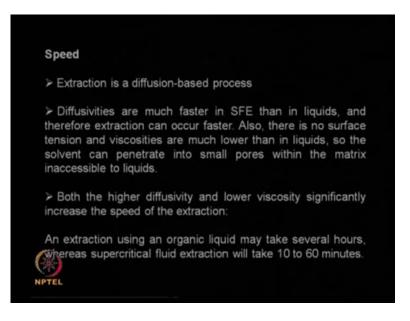
Speed, speed is very fast because, it is based on diffusion and as I showed in a few slides back, the diffusion coefficients are very high as against a diffusion coefficient of a liquid solvent. There is no surface tension and viscosities because, they are much lower than in liquids, the viscosity is much lower almost close to a gas, so it can enter very small pores, it can enter matrix and matrixes which are in accessible by liquids.
