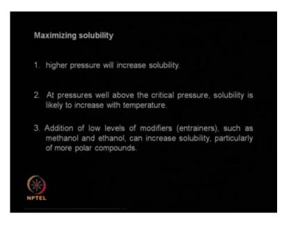
How do you maximize solubility, so we can use higher pressure when you use higher pressure solubility increases. At pressures well above critical pressures solubility is likely to increase temperature also, so if you are using very, very high pressure, than the super critical CO 2 temperature also may be very high. So, you may have to cool; that means, you need to put in an cooling system, to cool the super critical fluid.
