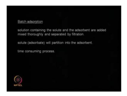
Now, let us look at different type of adsorption process; how a chemical engineering will look at? Because a chemical engineer is to process type of approach and we will look at different types of process. You can have batch adsorption, you can have continues adsorption and so on. What happens in a batch adsorption? What you do you take adsorbent and then you add it to a solution containing the adsorbate or solute which you need to adsorb; mix them both thoroughly.
