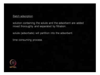
So, when you mix the adsorbent into the bulk your solute gets partitioned between the adsorbed and the adsorbent or in the bulk that your K; the constant value that com comes into the picture actually. So, this process is bit slow; it is a time consuming because it is need to do the adsorption. And, then it will do the desorption regeneration again you go back to the first step. So, it is a slow processes and time consuming.
