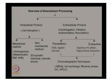
So, this is a nice slide, which sort of separates the intracellular products that means products inside the cell and the extracellular products that means when the product is in the media that is they are outside the cell. So, when you have intracellular product, of course, you have to disrupt your cell. That means you have to break the cells to get your product out, but if you are having intracellular product, you are not interested in the bio
