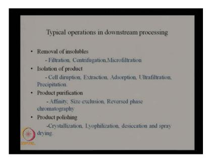
So, how do you remove insolubles? That means you are removing solid materials from liquids. So, there could be many techniques. We will spend time in the next course of the various lectures. Solids can be removed by filtration. They can be removed by centrifugation. They can be removed by membrane type of micro filtration, nano filtration, membrane filtrations and so on. So, all these techniques are meant to remove solid from the liquid.
