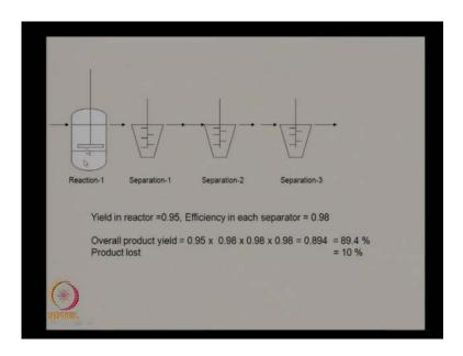
Now, let us go further imagine I have a fermentor or a bio reactor here and I am using three different separation steps. I am doing some separation in separator one. Then I am doing some other separation in separator two and then another separation in separation three. Each one of the separators has certain efficiency. It cannot be 100 per cent. It can be 98, 95, 90 and so on. It will be never 100 percent efficient.
