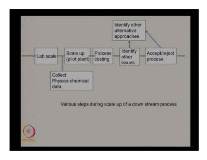
So, I talked about scale up. When we move from a lab scale, which is say about 100 milliliter scale, when you move to 1000 or 10,000 liter scale that manufacturing stage, it does not happen in one go. You need to consider several aspects when you are doing a scale up. So, this particular slide show you what are the various steps involved in scale up.
