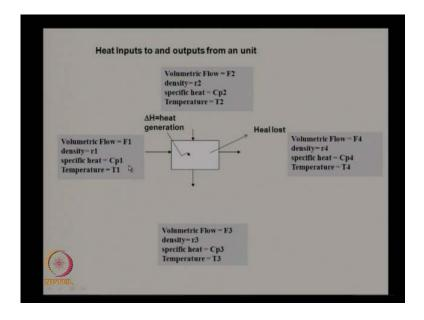
In heat balance, what happens is whatever heat that is coming in and there are heats going out. There are heat generated because of reaction or you are putting in some heat and there are going to be heat loss to the surroundings. So, there heat balance is slightly complicated. You are going to have many streams for heat balance. I think we will talk about this in next class.
