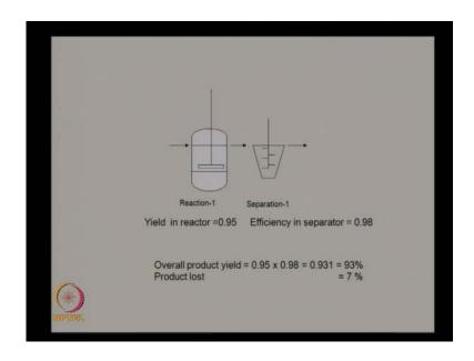
Let us look at the various issues that are involved in downstream unit operation. Now, let us consider. Imagine you have a reaction taking place in a reactor. It could be a bio reactor. It could be a fermentor. Then you are doing a separation, some type of separation, any type of separation you are resorting to and you are getting some product out here.
