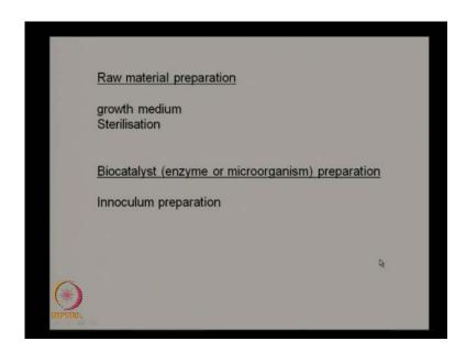
So, what is the raw material preparation? That is the left hand side, which we saw. We are preparing the growth medium. Growth medium means it may have a carbon source, nitrogen source, minerals, and micro nutrients, salts everything, which are needed for your growth of the microorganism. Then you need to sterilize all the growth media because whatever you feed into your fermentor has to be completely sterilized. So, this is what is called raw material preparation section.
