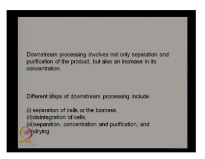
So, it not only involves separation, purification, but you are also increasing the concentration of your desired product like I talked about the alcohol fermentation after the fermentation from the fermentor, the amount of alcohol or ethanol in the broth may be 8 per cent, 9 per cent. But, finally, you want to make your concentration to almost 90 per cent. So, you are not only purifying your product. You are increasing it to very large concentration.
