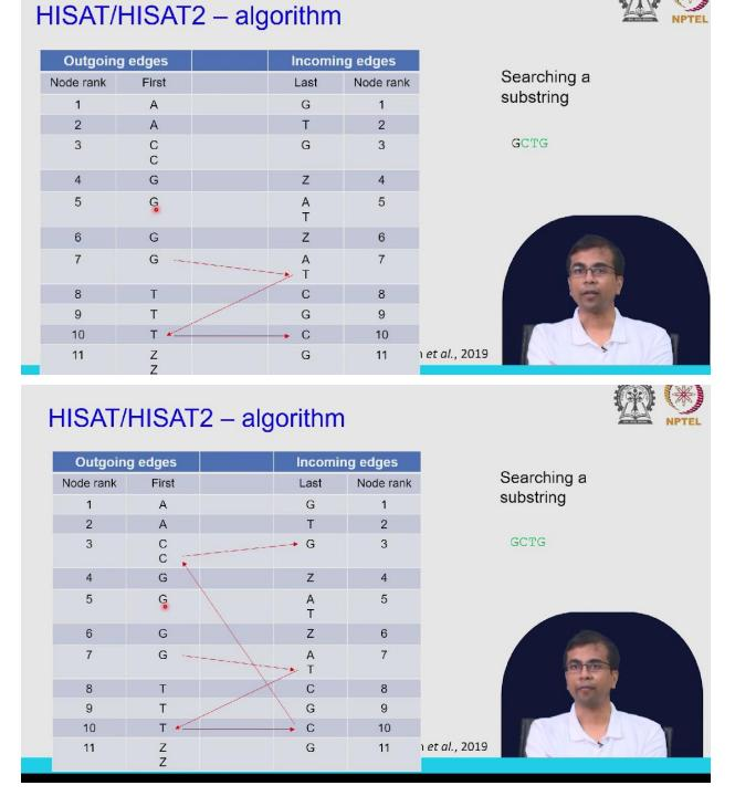
So, we can start with the last one, the G, and see where these G's are. So, these G's are here; their correspondence is given by these red arrows, and we can go to the last column right. So, which one is the letter that occurs before g? Remember, this is the principle that we had in the first mapping. So, the T is the letter that occurs before G, and we have found T here in two cases. So, we need to follow up on those two parts and this T because, because of the last mapping, they
