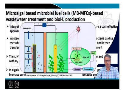
So, you can see here a kind of a schematic diagram is presented here where the waste water can be treated using the micro algal fuel microbial fuel cell to produce the hydrogen.
