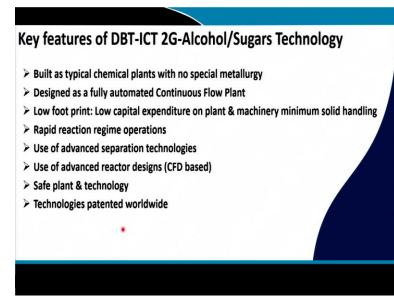
And the key feature of this strategy is or the technology is the built as a typical chemical plant with no special metallurgy. Designed as a fully automated continuous flow plant low footprint low capital expenditure on the plant and machinery minimum solid handling rapid reactor regime operation and safe plant and technology and technological technologies are patented worldwide. (**Refer Slide Time: 18:58**)
