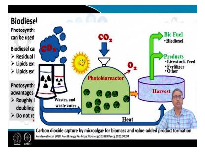
For example the carbon dioxide captured by microalgae for biomass and formation of value added product formation is shown in the diagram. Where you can see that the waste materials are used in the photobioreactor where further carbon dioxide is captured and then the biomass is produced which is converted into a kind of a livestock feed fertilizer and also the biodiesel molecules.
