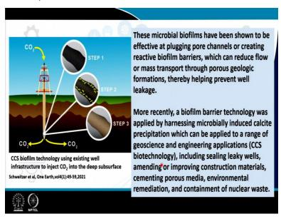
So, some of the aspects like the CCS biofilm technology, which helped in three steps like the microbial biofilm can actually allow in in effective plugging up the pore channels over there.
