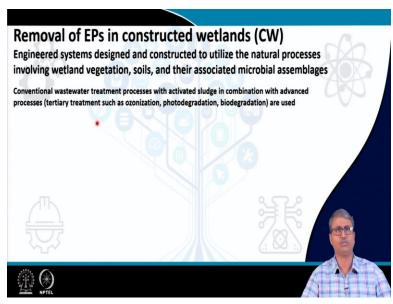
Now first we will discuss about the constructed waste wetlands. Now this is kind of an engineered system designed and constructed to utilize the natural process involving wetland vegetation, soil and the associated microbial assemblages. You can understand that the wetlands are being used for natural reclamation of the of the system or the natural treatment of the contaminated waste material waste water even.
