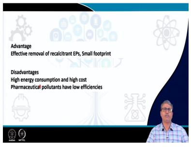
The advantage of this process is effective removal of the recalcitrant EPs and a very small footprint. Disadvantages include the high energy consumption and high cost pharmaceutical pollutants have low efficiencies for this.
