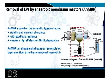
So, anaerobic membrane reactor system is based on the anaerobic digestion technology and is characterized by stability and microbial abundance, good toxic resistance and ensure high efficiency of the epibiotic gradation and it can also generate bio gas under anaerobic condition which is considered to be a renewable bio resource and it is in significantly larger quantities than the conventional anaerobic bio degradation system.
