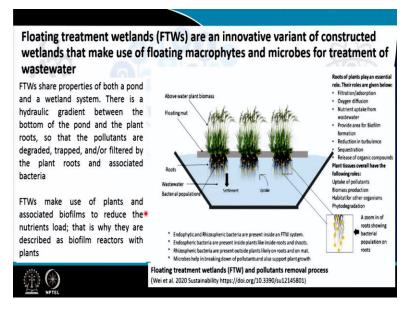
One of the most suitable technique is found to be the floating treatment wetlands are is kind of an innovative variant of constructed wetland that is making use and getting popularity. Because it is using the floating macrophytes and microbes in the water for treatment of the emerging pollutants present in the wastewater. So, as you can see here this is the water in which some mess is there and over this mess the plants are actually floating into that.
