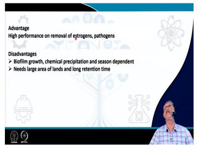
The advantage of this process is high performance on removal of the particularly what is observed for estrogen and different type of pathogens. The disadvantages are the biofilm growth chemical precipitation and season dependency needs large area of lands and long retention time.
