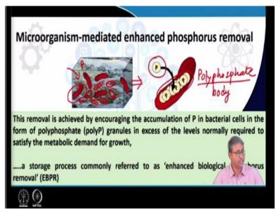
So, ideally if we look at the wastewater treatment process. So, this is for example the wastewater where we will allow the specific microorganisms to grow and once these microorganisms are able to encounter the phosphates which are present over there, so they will be able to accumulate the phosphate as polyphosphate body. So, these materials are called polyphosphate body.
