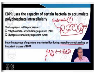
Now the EBPR the enhanced biological phosphorous removal process uses the capacity of these bacteria which are known as the polyphosphate accumulating organisms or conventionally also known as the PAOs. So, these PAOs are the organisms who are responsible for accumulating the
