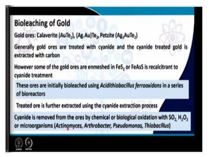
And finally the bioleaching of gold. Gold ores like Calaverite and Petzite etcetera are subjected to bioleaching. Generally gold ores are treated with cyanide and the cyanide treated gold is extracted with carbon. However some of the gold ores are enmeshed in FeS 2 or FeAsS is recalcitrant to cyanide treatment. And these ores particularly are initially bioleached because wherever the iron or arsenopyrite kind of stuffs are there.
