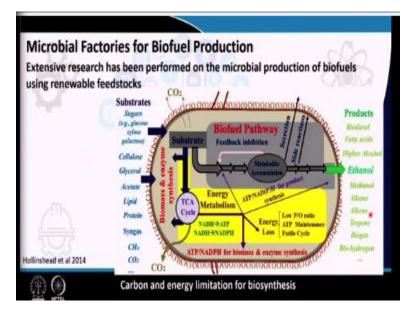
Feedstocks means, the resource which is provided to the microbial cells in order to gain the carbon and energy. Now, as you can see in this diagram, that a large number of substrates including the lignocellulosic biomass, the residues from the agriculture or the forestry or different products, organic products which might be produced from different other industries, including the food waste, or agricultural waste or food processing industries.
