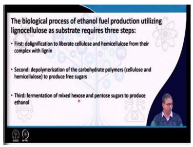
Now, the biological process of ethanol fuel production utilizing lignocellulose, as substrate requires three steps. The first step is the delignification, because it is a lignocellulosic biomass and we know it has very importantly the lignin as a important component. So, delignification is the first step to liberate the cellulose and hemicellulose from their complex with lignin. And the second is the depolymerization of the carbohydrate polymer that is the cellulose and hemicellulose.
