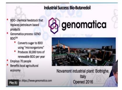
So, many industries are successfully implementing metabolic engineering. For example, the genomatica. So, genomatica has produced bio-butane or butanediol. Biobutanediol can be used for many purposes, where it can be a chemical feedstock that replaces petroleum based product. It is a raw precursor molecule for many compounds, which converts sugars into BDO that is butanediol through microorganism.
