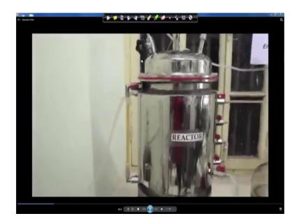
This is the bioreactor and you can see this is the watch glass and through the watch glass you can find out the volume of the liquid medium present inside the reactor and these are the other different units.
