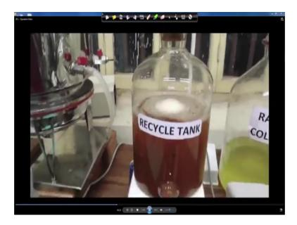
Where we take the liquid which is coming out from the reactor and recycle back to the reactor just to increase the retention time of the medium.
