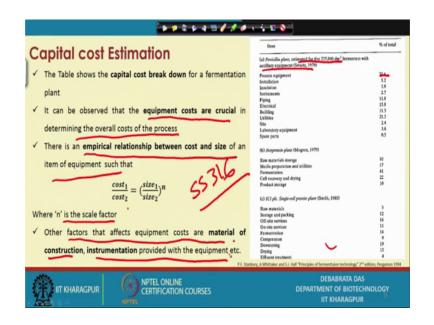
Now, capital cost estimation from the from the table you see that, this is the penicillin estimated of high 2 2 5 200 25,000 liter fermenter with auxiliary equipment, this is the this is the how this cost just percentage of the total is given, process equipment is 23.6 percent installation is 5.2, insulation is 1.9, in instrumentation instrument is 2.7, piping is 11.8, electrical is 15.8, building is 21 point. So, different cost distribution is given here.
