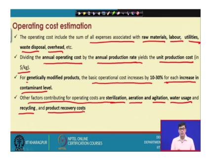
Then, operating cost depends on other several factors operating cost includes the sum of all expenses, like raw materials labor utilities waste disposal and overhead cost, dividing the annular operating cost by the annual production rate yield and unit production cost is the dollar per kg ah. For genetically modified product the basic operation cost 10 to 13 30 percent of the each increase in contaminant level.
