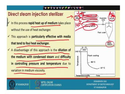
Now, direct steam injection because how it is done suppose this is the raw media am I right this is coming in this direction and this the steam is coming in this direction steam is coming this way and this is the mixing thing. And then this is this is called holding section, this is the holding and this is this is insulated this pipe is totally insulated so, that no heat loss take place.
