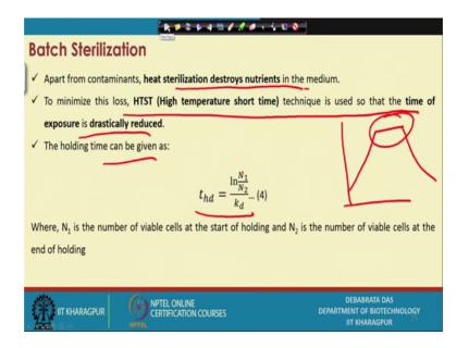
Now, this is the apart from the contamination the heat of sterilization destroyed the nutrients in the media, high temperature short time techniques is used. So, that the time exposure is drastically reduced the holding time we can holding time what is the specialty of that in the holding time you are melting the temperature constant.
