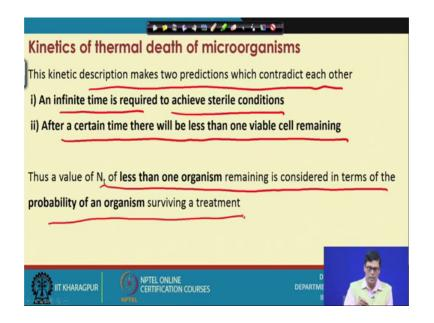
So, if you look at the kinetics description makes 2 prediction, which contradicts each other at a finite time at infinite time as the infinite time increase is required to achieve the steriliz sterile condition, and after certain time there will be less than one viable organism remaining, that is exactly I was try to point out that you know to get 100 percent sterility is very difficult to achieve.
