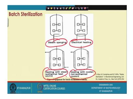
So, this is the major problem that we have I shall discuss more in details here and this is the device through, which we can we can do the batch sterilization one is steam and the electrical heating, and the heating will stream isolated heating source, and cooling with the coolant non thermal coolant, that we will different type of system we can use.
