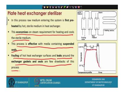
The, economy this is this economy this the steam requirement of heating and cooling the sterile is the media this process is effective with media, containing the suspended seals the seal fouling of the heat exchanger surface leaks around the heat exchanger gasket and seal fewer drawbacks of the process.
