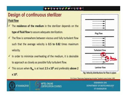
Now, we find that in the industry that up to up to 140 degree centigrade, we can usually use for the sterilization of the media. Now, flow characteristics of the media plays very important role, because if you know that there we have you know we have this is the plug flow, this is the turbulent flow, this is the laminar flow. Now, if you have this laminar flow you can see the velocity gradient act across the cross section of the tube.
