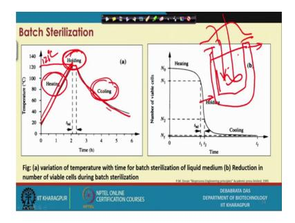
Now, this is the major problem that we have. Suppose this is the liquid am I right this is a liquid that present in the reactor and we want to heat it. Now, what we do that? So, suppose we can do it in two ways we can pass hot a hot a water here and increase the temperature this is the kind of started we have or we can inject the stream directly we can inject a we increase the temperature.
