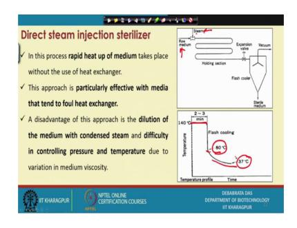
Because, if you look at here that you are what you are doing you are mixing media and, steam am I right as soon as you mix together the steam will undergo condensation as soon as the steam undergo condensation your media will be diluted and viscosity will be changed density will be changed as the, we know the flow characteristics of the fluid depends on the viscosity and the density. So, as they are changing. So, what will happen
