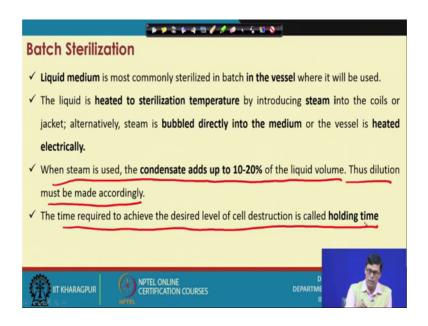
That, you know the liquid media is mostly is commonly this sterilized is sterilized in the batch vessel, where it will be used and the heated the sterilization temperature.
