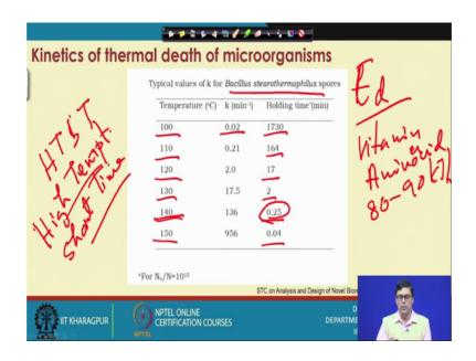
Now, this is the this is very interesting thing that if you look at here and a 100 degrees, if you are 100 degrees sterilization temperature k d value or the thermal death rate constant value k is the thermal death rate constant, the holding time is a 1 1 1730 minutes; that means, this is the sterilization time that is required. Now, a 100 10th degree centigrade it is required 164 degrees centigrade this is by using the organism bacillus stearothermophilus.
