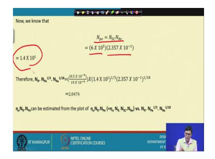
Now mu value is given here this is the mu is the viscosity of the air, and rho is the density of the air and the diffusivity of the air is given here. So we can easily calculate what is the Schmidt number Then we have the correlation that peclet number equal to Schmidt number into Reynolds number. So we have already found out what is the that that Schmidt number and Reynolds number. So our peclet number will come 1.5 into 10 to the power 5.
