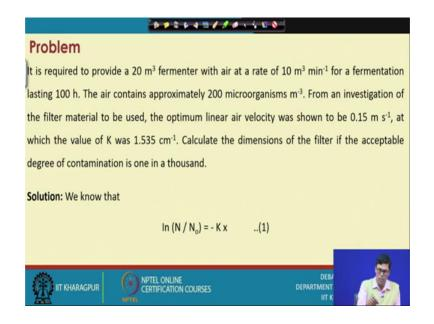
Now it is required to provide 20 cubic meter fermented with air at the rate of 10 cubic meter per minute for a fermentation, lasting for 100 hours the air contains approximately 200 microorganism part milliliter. Now from an investigation of the air material the filter material to be used the optimum linear velocity was shown 0.15 meter per second, at which the K value is 1.535 centimeter inverse.
