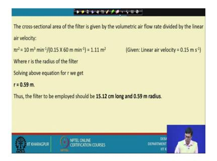
So r is 0.15 meter so we can easily find out that this is the per area now. Now where that where I the solving the above parameter then we can find out r equal to that then we can find out the r equal to that 0.59. So the cross section of the filter is coming about this radius is 0.59 meter and length is this the that we can easily calculate. That how we can we can we can do the calculation of this particular because I hope you understand that
