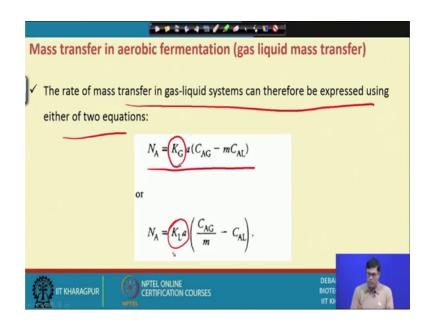
So, we can write that we have this equation that is the rate of mass transfer gas liquid system can therefore, is using the 2 equation, N A equal to K G a C AG minus m into C AL and N A equal to K L a C AG by m and on the basis of gas phase and the and the basis of liquid phase that, we can we can express this equation in the two way.
