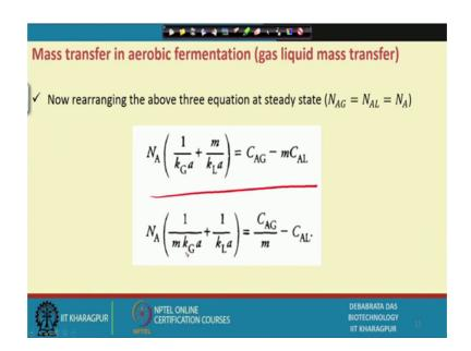
Now, rearranging the above equations we will we will come across this kind of correlation N A equal to that this N A into 1 k G a m by k L a C AG m into C AL and in case of other equation we can m a a a 1 by m k G a 1 by k L a you know C AG m by 1 into 1 this equation we can rewrite from that.
