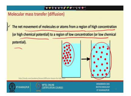
Now, what do you mean by molecular mass transfer, this is a very very simple example I have given, the net movement of the molecules or atom from a region of high concentration, or high chemical potential to the region of low concentration potential like this.
