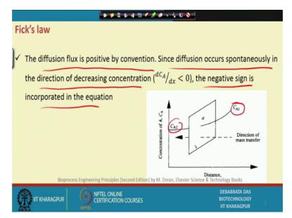
Now, this is the Fick's law; Fick's diffusion flux is positive by convection and, since the diffusion occurs spontaneously in the direction of decreasing concentration, the negative sign is in incorporated, this is the high concentration and this is the low concentration this is how the negative term has come.
