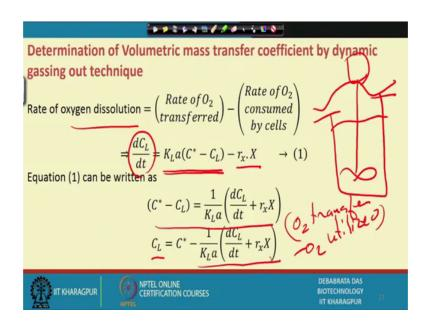
Now, this is the equation we can we can we can write, the rate of oxygen dissolution or rate of oxygen transferred, equal to that that rate of oxygen transferred minus rate of oxygen uptake by the cells. So, in a fermenter this is a fermenter so, two things simultaneously take place oxygen transferred one is o 2 transfer and another is o 2 utilize by the cell. So, the difference will get you, the how much oxygen that dissolve oxygen concentration increases in the system.
