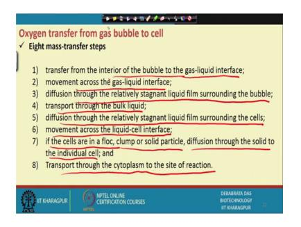
So, this can be written like this transfer from the interior of the bubble, then we are we can we can write the transfer of oxygen from the interior of the bubble, to the gas liquid phase and movement across the gas liquid phase diffusion through the relatively stagnant liquid film surrounding the bubble.
