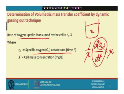
Now, rate of oxygen consumption how you can write that by the cell it is the r x is if we that, if we if we consider that suppose the if we consider the specific optic specific oxygen uptake rate, what do you mean by that 1 by x d o 2 by that means, gram of oxygen that that utilize per unit time per unit concentration of the cells.
