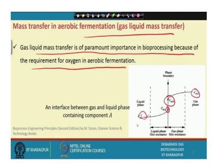
Now, let us see the how the transport take place mass transfer in the aerobic fermentation process, gas liquid mass transfer gas liquid mass transfer is the important in the bioprocess because, the requirement of oxygen in the aerobic fermentation I told you.
