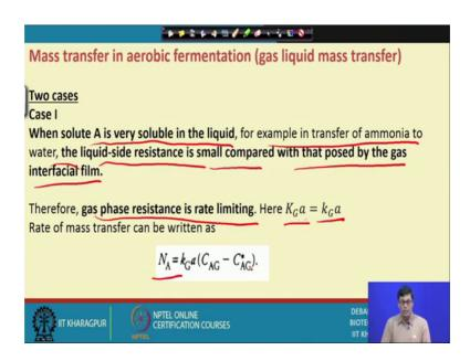
So, mass transfer in the has two cases a first case if you look at when a solution is very soluble in liquid for example, transfer of ammonia to water the liquid side resistance is small, as compared to posed by the by the gas interface because, where the solubility is more, then the resistance will be less therefore, gas phase resistance rate limiting is the K
