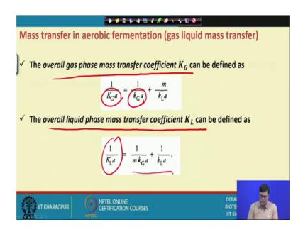
Now, these equation if you look at this equation that from this equation, we can write that one k this is this whole portion, what we can write this you can write 1 overall that overall, this we can write this overall gas phase mass transfer coefficient k G that is capital k G a not. So, this is small k G a and, this is capital this is overall.
