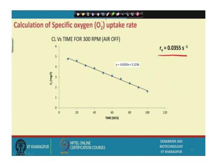
Then we find out the C L how the concentration of C L that decreases with respect to time that, we can find out this is just to find out the r x value, that we can we can find out that specific oxygen uptake by the cells, we can easily find out from this then we plot this.
