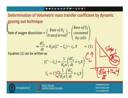
Now, here I want to point out that that in this that if you if you plot I just show you how you can plot that, C L versus this 1 d C L by d t plus r x into x. So, what kind of plot you will get negative slope this is negative am I right, this is negative slope and this slope will be what slope will be equal to 1 by 1 by K L a K L a.
