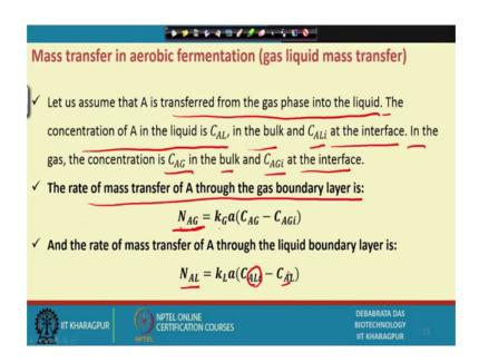
Let us assume a is the transfer a transferred from gas phase into the liquid phase. And the concentration of a in the liquid phase is C AL in the bulk in the bulk and C AL i at the interface, I showed you before and in the gas phase, it is C AG i n the bulk and C AG i is that the interface.
