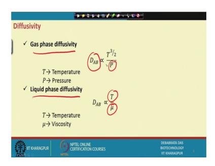
Now, diffusivity that depends on temperature that like this D A B A B is proportional to T to the power 3 by 2 by P. So, this is how this is gas phase diffusivity, another is the liquid phase diffusivity D A B equal to T by mu this mu is the viscosity of the liquid, here is the P is the pressure of the gas.
