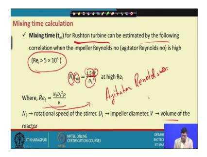
And this is applicable when Reynolds number is more than 5 into 10 to the power 3. Then this is the rotational speed of the agitated this is the mixing time equal to 1.54 volume of the volume of the layer reactor and Di is the diameter of the impeller. And Reynolds number is equal to D; this is this is called this is not the normal Reynolds number this is called agitator Reynolds number ok. This we call agitated Reynolds number.
