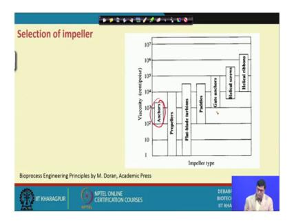
Now, if you use now viscosity plays very important role as per use of different impeller is concerned. Now, a anchor that usually lies in between 10 to the power 2 to 10 to the power 3 centipoises, then therefore, propeller is propeller, which is mostly used in the chemical industry that is 1 to 10 to the power 4 centipoise.
