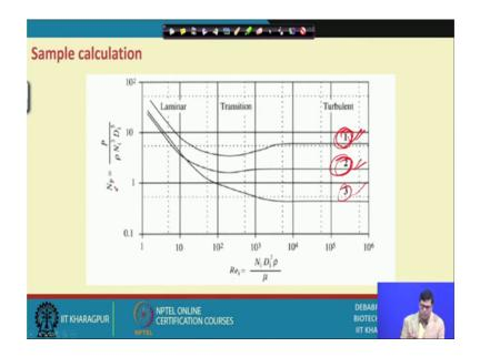
Now here I want to show you that that different region we have; we have laminar flow, we have transition flow, we have turbulent flow. The turbulent flow I told you it is lying in between 10 to the power 4 onwards, but in between approximately the 10 to the power 2 to 10 to the power 4, we have transition phase and laminar flow is the usually the Reynolds number 1 to 10 to the power 2.
