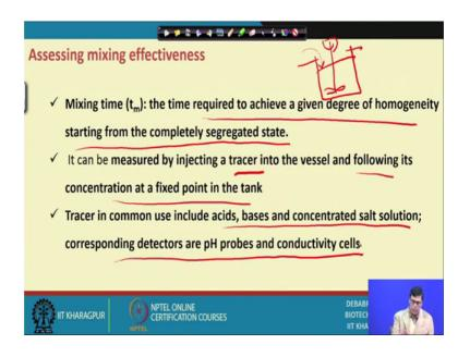
Now, mixing time who how you determine the mixing time is the time required to achieve given degree of homogeneity starting from the completely segregated state; that means, suppose this is this is a this is a liquid, and you put some material here. Now question come mixing time is the how quickly it is disperse into the medium; that means, how that time required for the homogeneity of the of the reaction mixture.
