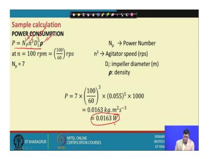
Now, similarly we can calculate also the power drown by the agitator, how you will; how can you do that power drown by the agitator is a Np; Np is the power number N the if the rotational speed of the stirrer, Di is the diameter of the impeller and rho is the density of the liquid. So, everything is known we put the value we can find out the what is the power drown by the agitator.
