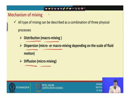
The mechanism of mixing; now what are the mechanism of mixing? Mechanism is mixing is the three: one is distribution dispersion, and their diffusion. Distribution we consider is the macromixing and dispersion it includes both micro and maximum unit depending on the scale of fluid motion and diffusion you consider as the of micro mixing. Let us see that what do you mean by that.
