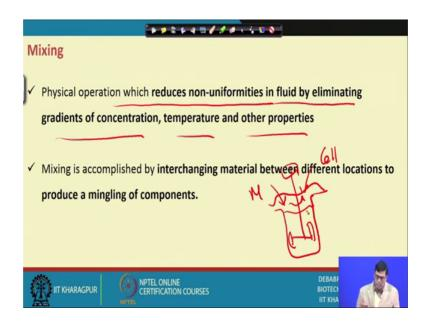
First let us know that is the; what do you mean by mixing? Mixing means that what we mean that; that which mixs the uniformity in the reaction mixture. As per example the physical operation which reduces non-uniformity in fluid by eliminating the gradient concentration, temperature and other properties.
