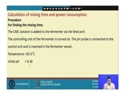
Now that for finding out mixing time, we put the CMC solution and they will maintain the temperature at 35.3 degree centigrade with the initial pH of 6.36.
