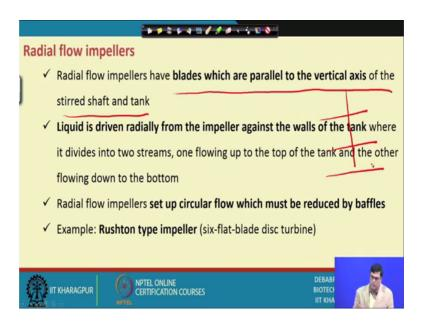
There are a different type of you know the flow patterns we have; one flow pattern we call it radial flow impellers; radial flow impellers what you mean by that?
