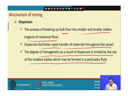
Dispersion is that the process are breaking the fluid flow if this smaller and smaller eddies. I have shown you only eddies, how eddies are created; region of rotational flow. The dispersion facility facilitates the rapid transfer of material through the vessel, throughout the vessel. And degree of homogeneity as a result of dispersion is limited by the size of the smallest eddies where which may be form in a particular fluids.
