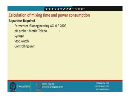
Next thing I want to share with you, that we guide out some kind of experiment in our lab, and just to find out that how to how to calculate the mixing time and how it correlated with power run by the agitator and the Reynolds number. Now we use the bioengineering AG fermenter and the pH probe; I told you whenever you do that you have to use some kind of monitoring device, and pH probe is required, then other things requires syringe, stop watch and other controlling unit.
