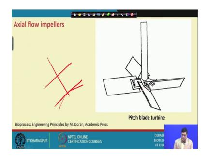
Now in case of previous thing it was perpendicular with this am I right. Now, here it is not the shaft; this blades are not in the perpendicular, it is kind of angle they are maintaining like this [FL] angle in there been maintaining like this.
