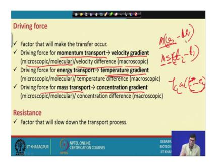
Now, that you know this driving force I can, we can explain like this, factors make again that the driving force is the momentum, transport is the velocity gradient, and microscopic it will be microscopic molecular and velocity difference. This is the momentum as I understand that mass into velocity am I right; also it is the mass is the velocity gradient that plays very important role.
