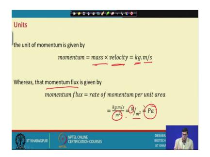
Now momentum as I pointed out this is equal to mass into velocity, what is the unit of mass kg. And what is the unit of velocity that is mass per unit time.
