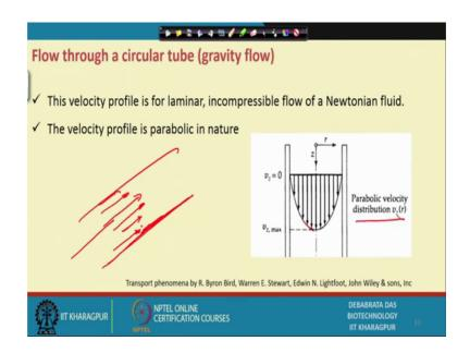
Now, flow through the circular tube the velocity profile in the laminar, of a incompressible liquid Newtonian flow, this is the this is the velocity profile with a what I want to show, this is suppose the liquid is flowing through this pipeline. So, it will be having like this. Now, why because you know this is exactly 45 as the liquid comes close wall of the tube, there will be friction between liquid and the and the and the wall.
