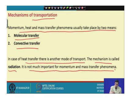
As I point out the interesting that mechanism of transportation that momentum, heat and mass transfer phenomena usually take place by two different means: molecular transfer, and what you call convective transfer.
