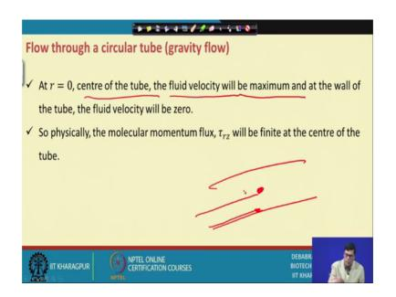
So, flow through the size circular tube, what is happening; if r equal to 0, if r equal to 0, center of the tube, the fluid velocity will be maximum. Suppose, this is the tube and you know that; if the velocity is the maximum here, why it is velocity; where you have less friction as you come to the close to the wall there will be friction between wall and the liquid.
