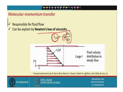
Now, molecular momentum, if you transfer; how you can calculate. Suppose, there is a two plates this is the two plate, this is one plates and one plates the water is there stagnant water is there. Always suddenly you move this bottom plates, then what will happen; the velocity of the lower fluid will be like this, it will be the profile will be like this can explained that with the help of Newton law viscosity this is the shear stress am I right and this is a shear rate.
