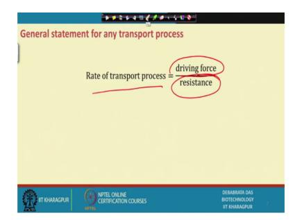
Now, general statement of transport processes. Now how you can do that? Rate of transport process is the driving force blindly defined by resistance. So, you know driving force means, suppose you know you want to heat some liquid; now what is the driving force? Driving force is the temperature difference and resistance is the media that you know they hinders that you know that that um that flow of the, that heat. So, you know that.
