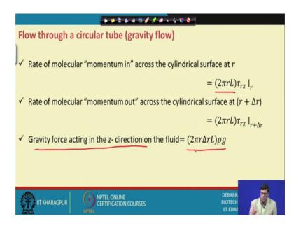
Now, rate of molecular momentum in can be explained like this. This is the surface area, am I right; this is per unit surface area. So, tau r z this is r, then this is r plus del r and this is the gravitational, this rho g you multiplied you will get the gravitation force acting on the z direction of the fluid.
