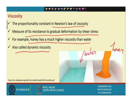
The viscosity is the proportionally constant of the Newton law of viscosity. Measurement of resistance is gradually deformation of the shear stress. For example, honey has much higher viscosity then water and also as dynamic viscosity.
