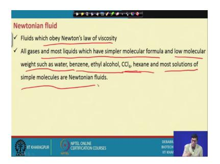
Now, Newtonian fluid, what do you mean by Newtonian fluid, which obeys the Newton law of viscosity. That all gases most liquid which have simpler molecular formula and lower molecular weight such as water, benzene, ethyl, alcohol, carbon tetra chloride, hexane and most solutions of simple molecules are Newtonian fluids. So, this is this is how Newtonian fluid can be defined.
