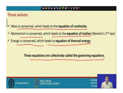
Now three axioms are there mass is conserved, which will lead to equation of continuity. Momentum is conserved, which leads to equation of motion and energy is conserved, which lead to equation of thermal energy.
