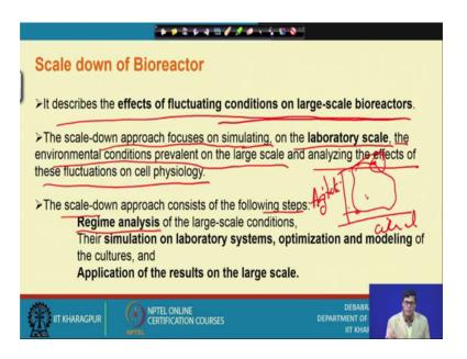
Now, in the scale down what happens is described scale down is when you describe effect of fluctuating condition on the large scale bioreactor because, you know that that a you know when we operate any kind of fermenter it may so, happen that you know operational condition may change you know the although, I can give their it simple example that power failure power failure is a common issue, of any kind of industry as per India is concerned.
