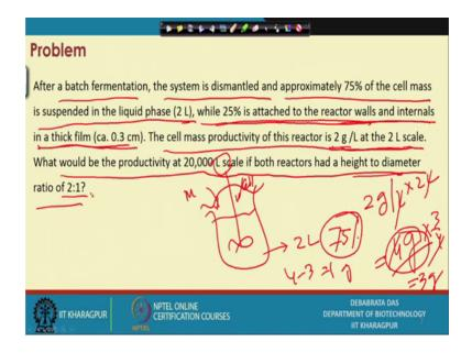
Now the problem says after a batch fermentation the system is dismantled, dismantled means the you just open it up and approximately 75 of the cell mass is suspended in the liquid phase that is the 2 liters, and while 2 percent attached to the reactor wall and internal with a thickness of calculated 0.3 centimeter.
