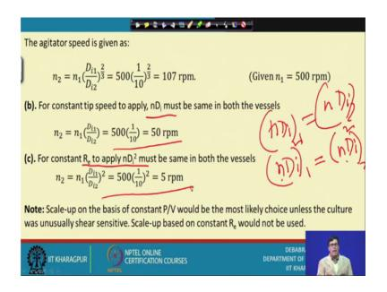
Now next problem that we have that is if when that tip for the constants tip velocity, constant tip velocity means n D i 1 is equal to n D i 2.
