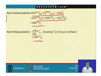
And then finally, we want to find out that; what is the amount of gas produced. The we have already developed this equation that 0.35 into E E Q is S 0 1.4 to in to P x, all the parameters is already estimated. So, we can find out 1408 cubic meter methane produced per day.
