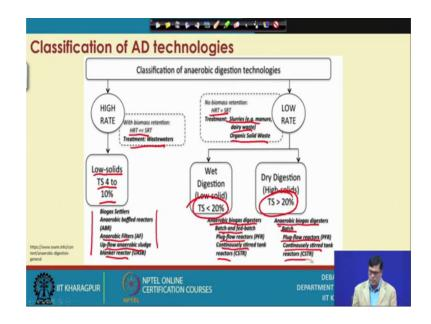
Now classification of anaerobic digestion technologies, this can be we can we can we can we can classified at the high rate and low rate. High rate this you know that hydraulic retention time is less than a solid retention time and with the treatment of the waste water. This is the low solid content that total solid a 4 to 10 percent with use at the biogas settler, anaerobic baffled reactor, anaerobic filter up flow, anaerobic sludge blanket reactor, these are the different reactor is use.
