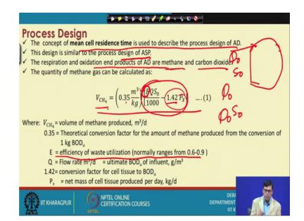
Now, if you look at this you know, this is very important the process design of this process that a concept of mean cell residence time is used to describe the process design of, we say we already explained that what is called mean cell residence time and design in similar to the activated sludge process respiration oxidation in product of anaerobic digestion or methane and carbon dioxide. The equation is V into this is very important.
