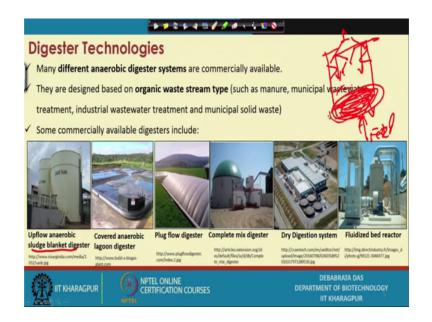
Now, we have we different anaerobic digesters is commercially available throughout the world and this is the up flow anaerobic sludge blanket reactor, up flows sludge blanket reactor appears to be the very efficient reactor. Now what is that reactor. This is the reactor is like this and. So, here we have we have some kind of sludge that here we have this.
