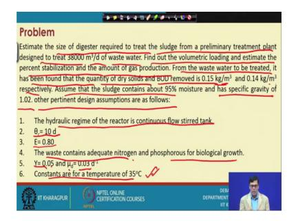
Now, we have we have taken one problem that you know they, estimate the size of the digester required to treat the sludge from a preliminary treatment plant design 3 38000 cubic meter per day of wastewater. Find out the volume loading and the estimate the percentage stabilization and amount of gas produce. From the wastewater to be treated, it
