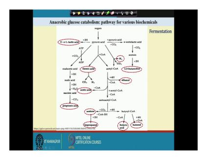
So, different type of antibiotics, how it forms it has been shown here. Then other Anaerobic fermentation process, we get different type of various chemicals we can get like Propionic acid, isopropanol, butyric acid, butanol, ethanol which now, it is plays very important role. Because as the source of energy and particularly Lactic acid is largely used for the food preservation purpose. So, it is used in the food and farm food and pharmaceutical industries and poly lactic acid is used.
