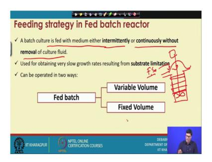
Fed batch process means, that the batch culture that is fed in the media, either intermittently or continuously without removal of culture fluid.
