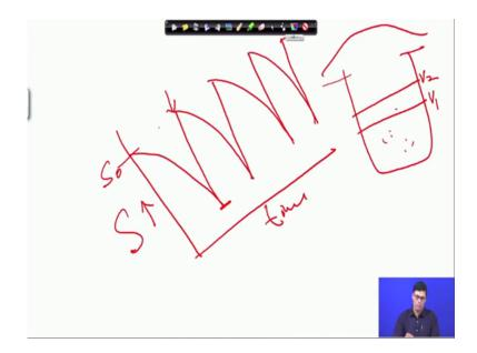
The substrate concentration will keep on decreasing, suppose in this reactor you put the your raw materials then, allow to react, then what will happen? That substrate concentration will decrease with respect to time. When it is comes to minimum, then again you feed it. So, this is you can increase the feed like this.
