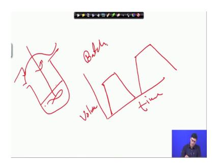
Suppose, what I am saying that this is the reactor. Now, this is moving like this. Now, when you consider the batch process, how you; how what is the basing the feeding strategy we have? Like this. We take the material allow it to react, and then take out the
