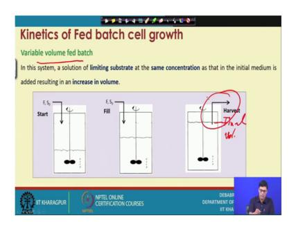
Now, here, we have given the example of the variable volume fed. So, we start with this volume because, this is the start then we increase little bit, you can see that below and final volume (Refer Time: 06:40) then, when there is the final volume this is the final volume, am I right? Final volume when is reaches the final volume then, we do the harvesting of the material.
