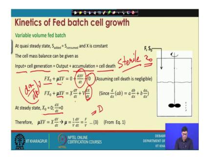
So, this will be dx by dt into V, am I right? This is the volume will be take place the output will be 0, there is no output in the fed batch reactor and rate of accumulation everything is the accumulative in the system cells are accumulation, can be expressed like this, and we can we can assume that, there is no cell death occur in the system.
