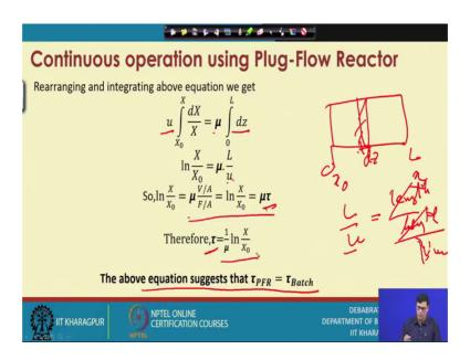
Now, if you do the integration that, you know that u is the velocity and d X by X u will be d z. And so, this is the reactor that we have a strip here. So, this is d z. This is the length is d z.
