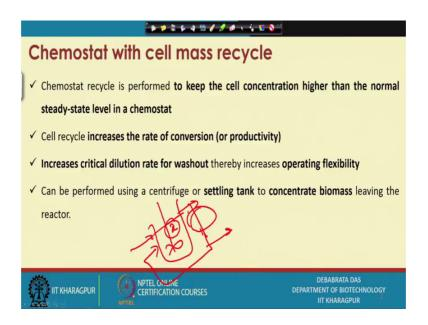
Now, this can be overcome. How you can overcome? This can be overcome, suppose, the whatever x s s cell mass is going, so, if you put a separator here and we can and part of the cell, you are recycling back to the system to maintain the cell mass concentration uniform, then and all then your rate of reaction will be constant. Then there will not be any problem of cell washout. So, this we will discuss here.
