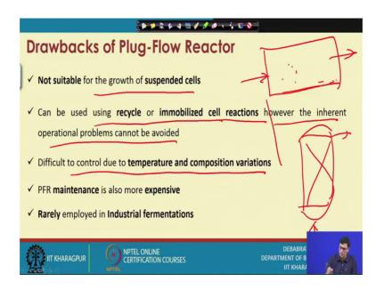
The drawbacks of the of the block flow reactor, it is not suitable for the growth in suspension because, I told you that in the plug flow reactor, there is no back mixing.
