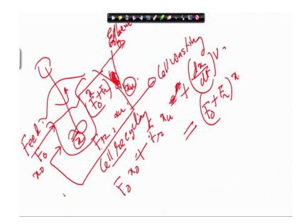
So, if we see that you know that C S T R of the cell mass recycling system, it basically looks like this. So, this is rotation; this is like this. So, here we can have the settler and this is going out and part of the things you recycle back and part use. So, here what you call cell recycling, this is recycling. And this is called cell wasting.
