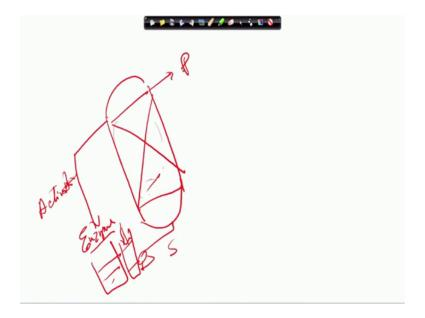
Suppose, this is a solid this is a column and inside this column we have any kind of solid matrix we can put it, we can as for example, I we can use any we can use coconut coir. Coconut coir is a fine fiber, so, we can pack the column. Why we use coconut coir because it has more lot of surface area. So, more surface area more will be the immobilization of enzyme.
