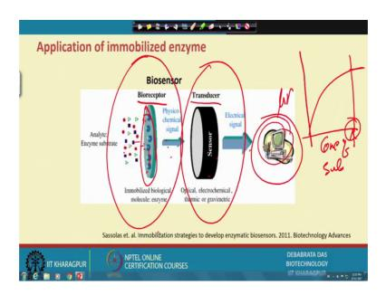
Now, as I pointed out that one important application that we have is the biosensor. Now, question come how biosensor they are produced. Now, here in this picture, you will find that that two part is there one is this is bioreceptor, and this we call molecular recognition unit, and this is called transducer. So, you know it has it divided into two different parts. One is molecular recognition unit; another is transducer. The molecular recognition unit that mean part for to recognise the molecule.
