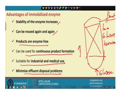
Now, advantage of the immobilized system that first with the stability increases that already we pointed out can be reused again and again that also I pointed out. So, suppose in a big column, so you can put your immobilized enzyme here, and here you pass suppose you want to produce glucose, glucose to fructose, the glucose isomerase enzyme glucose isomerase, so you immobilized that immobilized glucose isomerase here you will get the fructose.
