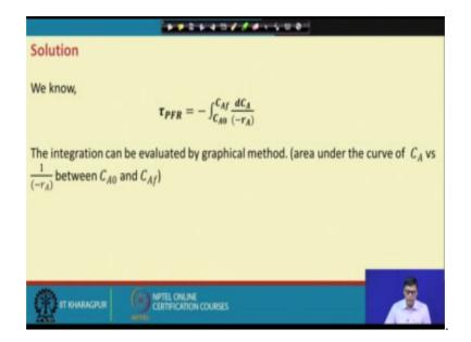
Now the equation is that equation for this is the tau plug flow reactor is this and the same as your batch reactor the integration can be evaluated graphically under the carve C A versus 1 by R C A 0 to CAF.
