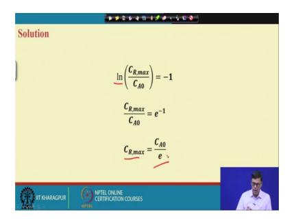
Then if this is equal to minus 1 then this is like this then then C R by C max equal to C A 0 equal to C A 0 equal to this ln is there. So, ln I can I can I can ln if we take it ln out that C R max by C A 0 equal to e to the power minus e 1 and C R max equal to C 0 by e. So, this is how we can we can solve this equation in other approach, but I feel that the first
