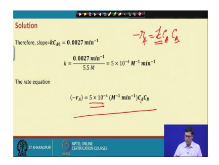
The once we get this k value then we know our rate equation what is our rate equation minus r A equal to k into C A by C B am I right. So, k now k value has been determined. So, we can put this k value here and this is how we can write the rate equation and again I am telling you if you want to do the validity of the equation, we can easily do by ourselves in that case we shall have to find a correlation between the time and the and the
