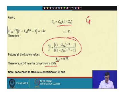
Now, once that here we have this equation then we at the same time we know that C A equal to what C A equal to C A 0 into 1 minus X A at any point of time. So, in this equation you can put the value of C A then we have this equation and then for different temper to different time because the t 2 and t 1 if the fraction the 1 time X A 1 is converted and their time 2 X A 2 is converted that we can have the expression is like this.
