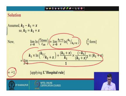
Then again we can we can have we can assume k 2 minus k 1 equal to X k 2 equal to k 1 plus X then we can write this equation in this form and then if we solve applying this law hospital rule then we will get this is equal to minus 1.
