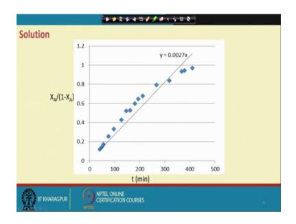
So, this is this is exactly that from the slope we can find out that value of k we can find out and this is how the k value is coming around this now.
