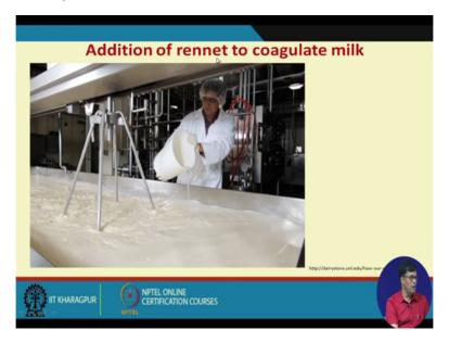
Then addition of rennet that for coagulation of the milk that rennet is kind of soluble in water we add here rennet for precipitated out the proteins.
