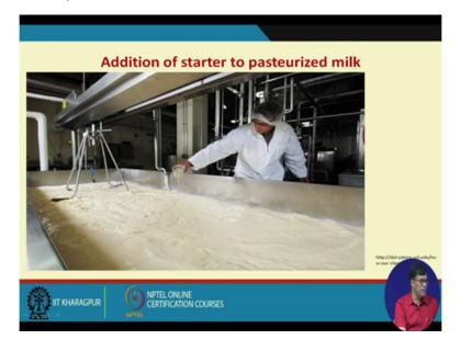
Now this is addition of starter in the milk you can you can in the pasteurized milk we can add the starter here, this is the milk and this is usually done in a vat.
