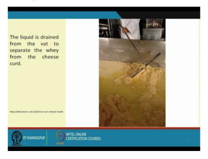
Now liquid that is you know this is now you can see the grain size here how the solid particles is separating out from this you can find out this liquid is drained that fat to separate the whey from the cheese curd you can see how it is this is the liquid and this is the solid that we have.
