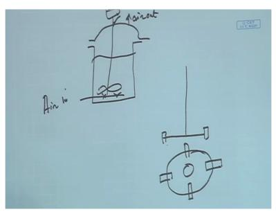
Impeller to mix the culture evenly, so it is the use the impeller, impeller I have already shown you how it looks the impeller it is like this and if you take that you know the top view or bottom view it is like this, the disc, in the disc this is centre point and the this is the blades are mounted like this, so this is rotate like this and this is called impellers.
