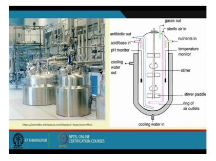
And this is the fermenters and this how the impellers (())(019:21) looks. There is the different type of fermenter that is used we have we can have this in different air in I showed you there is the air-in and this is air-in and air- out, this is that we have. Air-in here and air-out gas-out that is temperature monitoring system that we have.
