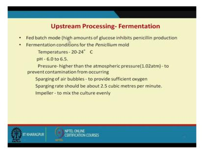
So this reactor fed batch reactor was found most suitable for the penicillin fermentation process because substrate here substrate acts as a inhibitor. After that is after the end of the fermentation pH is rises to 8. Fed batch mode high glucose inhibition of penicillin production takes place that can be taken care by using the fed batch reactor. The fermentation condition is 20 to 24 degree centigrade, pH 6 to 6.5, pressure higher than the atmospheric pressure 1.02 to prevent the contamination.
