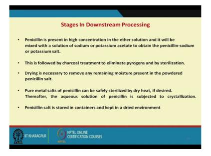
And penicillin is present in high concentration in the ether solution is being mixed with a solution of potassium or sodium acetate to obtain the penicillin or sodium salt of penicillin. So you know we can penicillin-sodium or potassium salt we can produce if we use the sodium salt or penicillin potassium salt then we get that. This followed by charcoal treatment, because we have seen that charcoal have some bleaching this eliminate the pyrogen and by sterilisation process.
