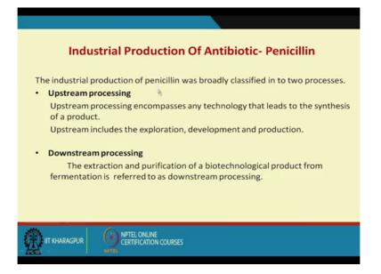
Now industrial production of antibiotic penicillin; industrial production of penicillin broadly classified in 2 processes, one is called upstream processing. Upstream processes encompass any technology that leads to the synthesis of product, then the upstream includes the exploration and development and production and downstream processing basically the extract, purification of biotechnology product from the fermentation is referred as a downstream processing.
