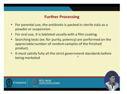
The further processing for parental use, the antibiotic is packed in a sterile vial as a powder suspension. For oral use, it is tableted using the film coating. Then searching test for purity potency are performed on appreciable on the appreciable number on random sampling of the finished product. And it must satisfy fully the strict government standards before being marketed.
