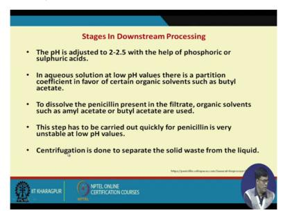
Now after taking out this as I told you, the pH is adjusted to 2 to 2.5 with the help of phosphoric and sulphuric acid and then in the aqueous solution at low pH there is the partition coefficient in favour of certain organic solvent such as the butyl acetate, amyl acetate. This they show as you when you reduced the pH, the partition coefficient will be that is solubility of solute will be more in butyl acetate as compared to the aqueous layer.
