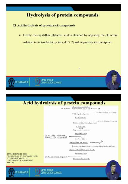
Now, finally the crystalline that glutamic acid obtained by adjusting the pH of the solution with the isoelectric point pH 3.2 and separating the precipitate. This is the finally we can separate out particular this glutamic acid like this. Now if you look at the steps involve in this particular glutamic acid for that process from protein hydrolysis, so we take gluten, soya bean cake and casein.
