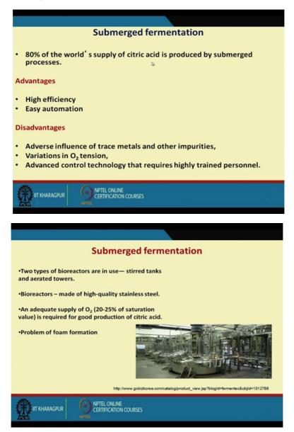
Now 80 per cent of the world's supply citric acid is produced by the submerged fermentation process it is considered as a highly efficient and easy automation. This advantages the adverse influence of the trace metals and other impurities and variation of oxygen tension, advance control technology that require high trained personnel , because because this is the kind of since it is the fast process so you require little bit trained personnel for the operation of this process.
