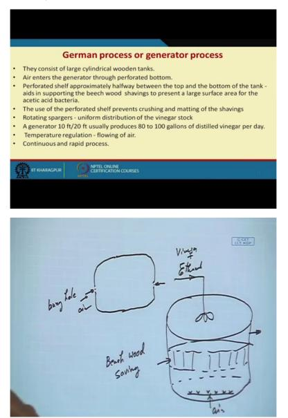
And this is consists of large cylinder, wooden tank so I can give the example that this is the wooden tank.
