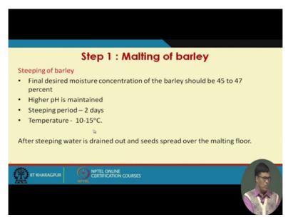
After the steeping process the final desire is the moisture concentration of the barley grains should be 45 to 47 per cent, pH higher pH is maintained and steeping period usually for two days and temperature we maintain 10 to 15 degree centigrade.
