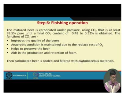
Now finishing operation the matured beer is carbonated under pressure using the carbon-dioxide that is at least 99.5 per cent pure until final carbon-di-oxide content is 0.48 to 0.52 per cent is obtained. The function of carbon-di-oxide is several it improves the quality of the beer because beer is a carbonated drinks and I told you this this this protein helps for maintaining the foam in the beer.
