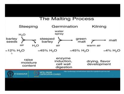
Now it can be explained like this the steeping process barley grains in presence of water. This initially the water contents the barley grains is 12 per cent then when you soak in the water the this barley grains water then it increase to about 45 per cent and then this barley grains we keep it I told you that we keep it under aerobic conditions and under humidified condition so that the germination takes place.
