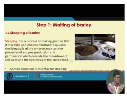
Now steeping process is looks like this soak in the water you can see how it is there, it is a process of soaking barley grains so that it may take up sufficient moisture to quicken the living cells of the embryo and start the process of enzyme production and germination of the which precede the breakdown of the cell wall and the hydrolysis of the stored food. This is undone in the aerobic conditions.
