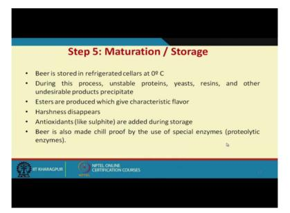
Now maturation process I told you I mentioned before the beer is stored at the refrigerated cellars at 0 degree centigrade and during this process unstable protein yeast and resins and other undesirable proteins are precipitated out which is very important.
