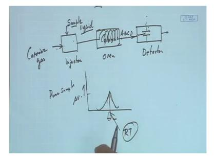
So maybe we have some micro volt here that change of microvolt, this we correlate with the kind of concentration of the component present in the sample. This is the visual output that we have the separation different peaks and patterns of the chromatogram corresponds to the different components of the of the separated mixture.
