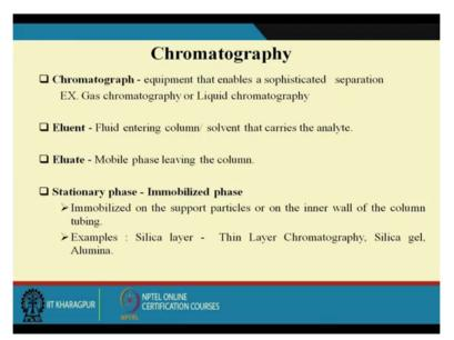
So this is largely used this is called gas chromatograph. In the liquid chromatograph this mobile phase will be liquid so here the only the advantage of this of this liquid chromatograph that we can analyse both the volatile and non-volatile component present in
