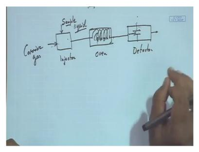
So in case of gas chromatography we can we have three different section one we call injector this is called injector and another we call oven where we have column and another we have detector. So what you do here we put the sample measured amount of sample with the help of syringe then here we put the carrier gas, now here everywhere we can maintain the temperature we have different temperature control here we maintain temperature here everywhere you have heater you can maintain the temperature.
