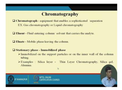
Now chromatography we have the chromatography is equipment that enable a sophisticated separation as for example we have gas chromatography, we have liquid chromatography. The basic difference between the gas chromatography and liquid chromatography is that mobile phase in case of gas chromatography is the gas. So we use gas as a sa a carrier because when we inject the sample and then it vaporizes.
