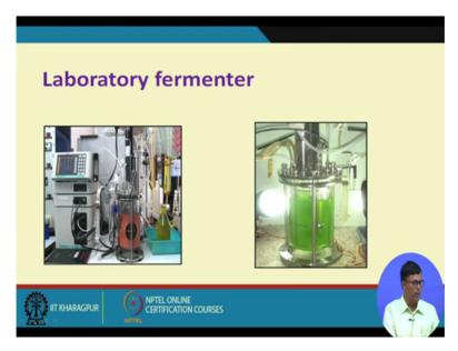
And this is another fermenter we have. This is New Brunswic fermenter that also this is the control module control module and this is the this is the fermenter that we have different parameters that is we stayed here you can easily visualise that what are the values of the
