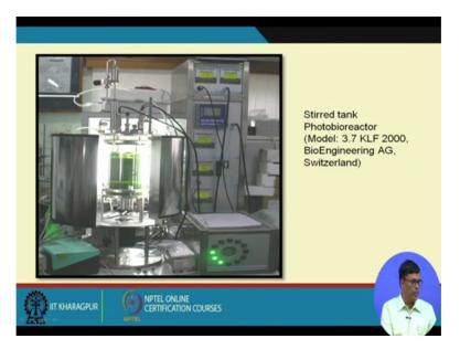
Now this is the bio engineering fermenter that is in operation in my in our lab. You can see this is the control control module. Where we can monitor different parameters live. We can monitor temperature, we can we take admission paid, then ph of the Seasons, dissolved oxygen concentration all this thing you can monitor this process that you have different monitoring system that we have here.
