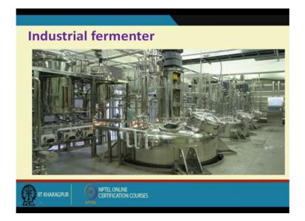
Now as I told you I work with citric acid industry and our capacity of The vessel was 200 cubic metre so that the power drawn by the power required but the is it it was around 200 HP is very high very huge amount of power we usually apply. So this and this power if you directly applied to the sat we can imagine what should be the velocity of the visitation speed will be driven the size. So what you what you do for first we put put the power in the gearbox.
