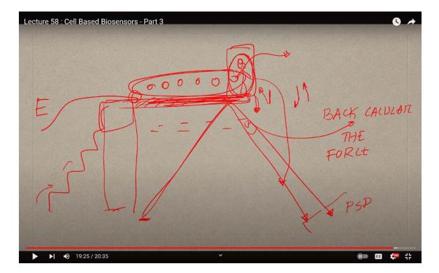
Now, imagine applying this principle on a much smaller scale. In a microcantilever array, each cantilever functions like a tiny diving board. If we could grow individual muscle cells on top of these cantilevers, we could measure the force generated by those muscles.
