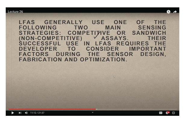
In essence, the process involves a surface coated with highly specific binders. When a sample is introduced, it flows across this surface. If the sample contains an antigen that matches the antibody on the surface, binding occurs. The speed at which this binding happens can be crucial, as the bound antibody typically carries a marker, this could be a
