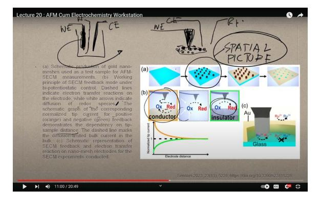
In this advanced setup, the AFM tip itself can function as the reference electrode. As the AFM tip scans the surface, it detects various properties. If the surface is conductive, the AFM tip, which can be modified to act as a conducting electrode, can sense and measure
